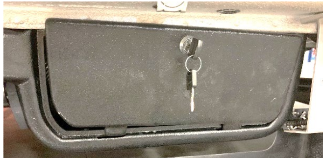
35.5 Locking storage compartment for flexible macerator hose
