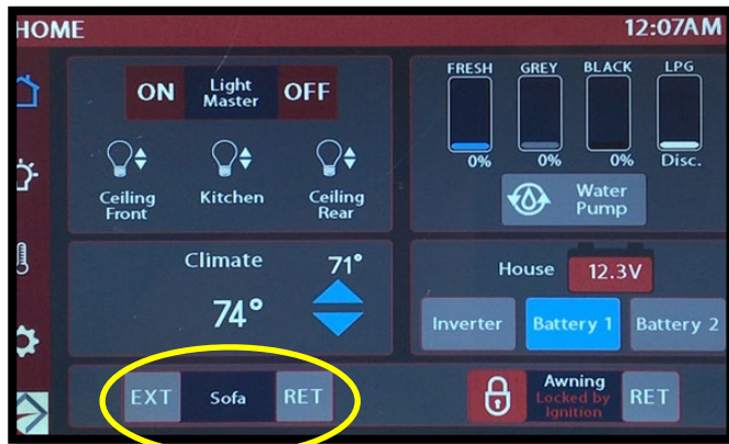
20.2 Sofa controls on monitor panel
