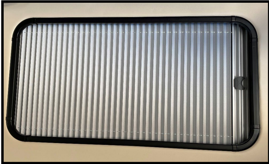
20.1 The side window screens – nightshade side
