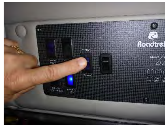
Picture 42.2 Water pump switch
