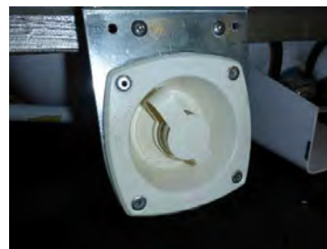
City water connection with built in pressure regulator
