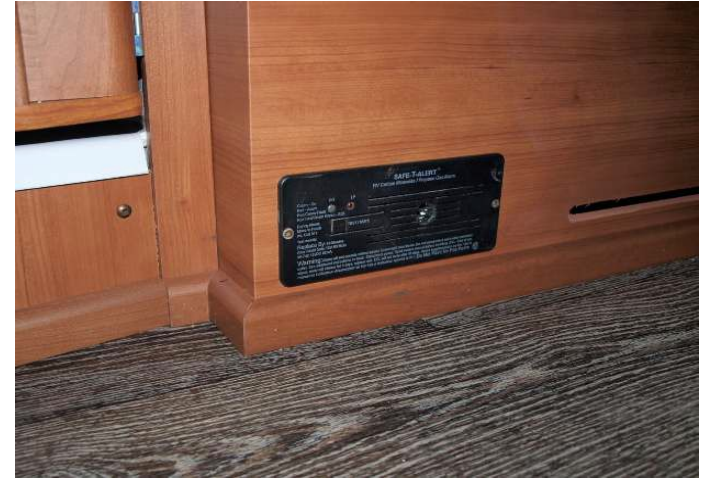
Propane and Carbon Monoxide alarm
