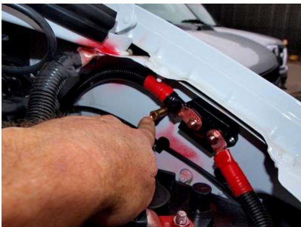
Coach batteries and negative jumper attachment point – brass stud protruding from side wall of engine compartment
