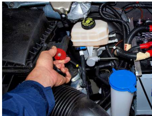
Positive jumper point, on driver's side of the engine. Red disc is pushed back to expose the contact
