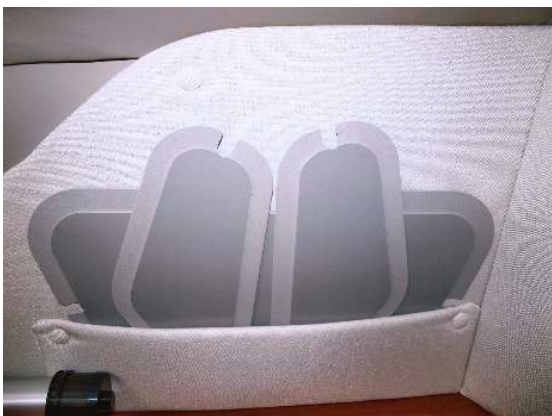
Picture 23.3 Skylight cover storage
