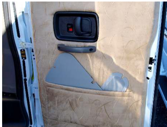
Picture 22.3 Skylight cover storage
