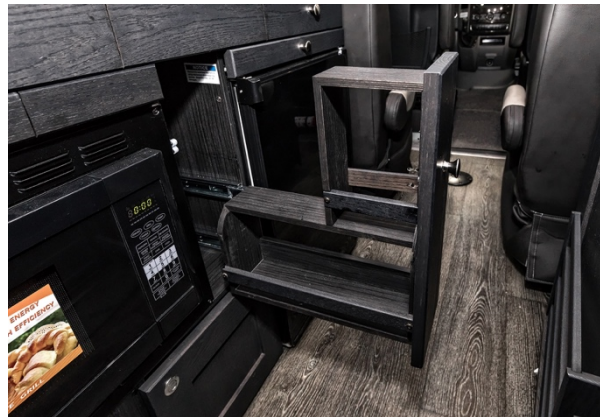
Picture 17.5 Slide Out Pantry Located Between Microwave and Refrigerator.
