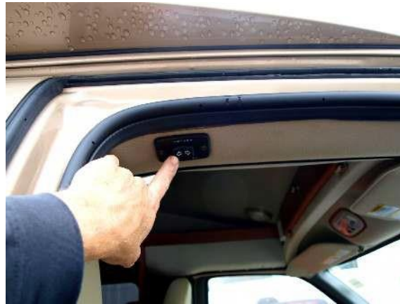
Awning power switch
