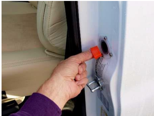
Exterior tank fill location (driver's side door pillar)
