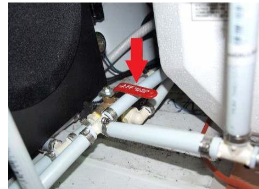
Tank selector in interior tank position
