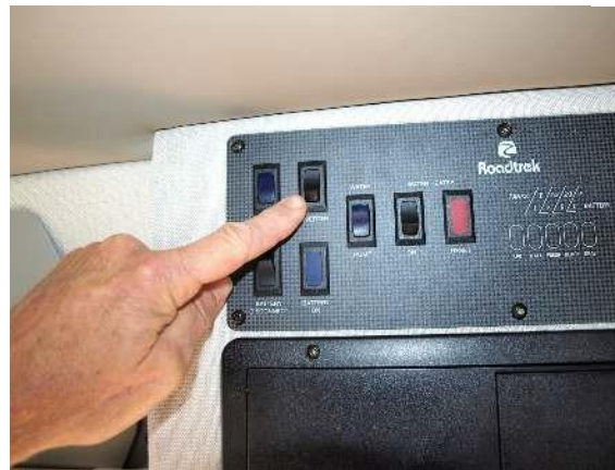
Inverter switch for standard 750 watt inverter
