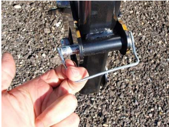
Spare tire retaining pin
