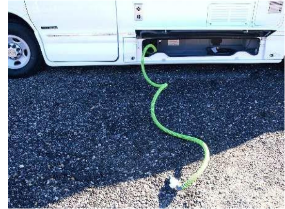
Driver's side center access door houses power cord and waste discharge hose
