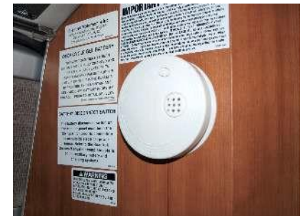
Propane and Carbon Monoxide alarm
