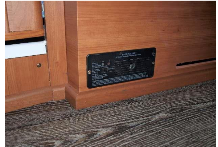
Propane and Carbon Monoxide alarm
