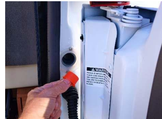
Interior tank fill location (rear door, right side)
