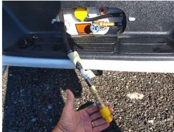
High pressure BBQ pigtail
