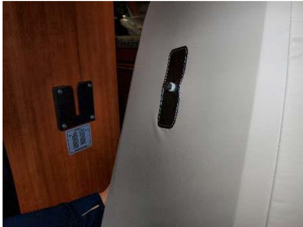
Second row seat back pin and slot
