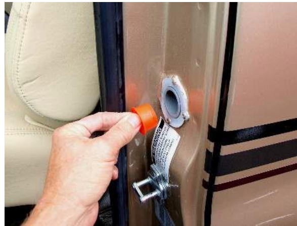
City water connection for hooking up to pressurized water
