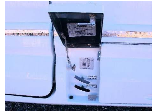
Driver's side front access door showing tank dump valves
