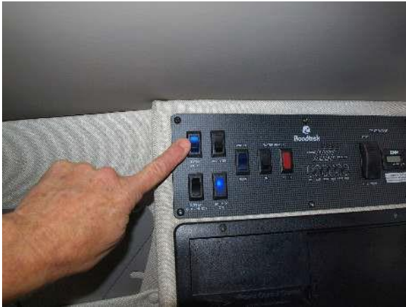
Patio light switch
