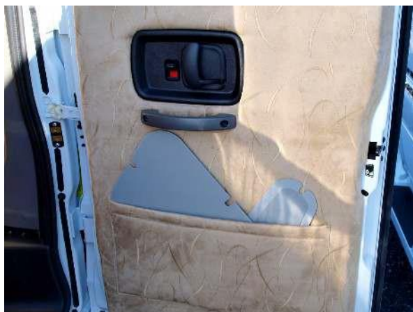
Skylight cover storage
