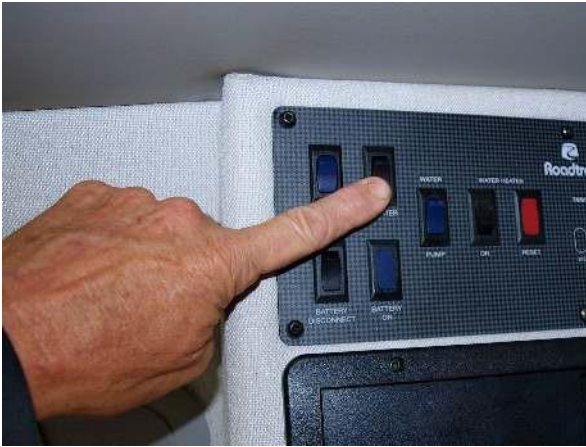
Inverter switch with standard 750 watt inverter
