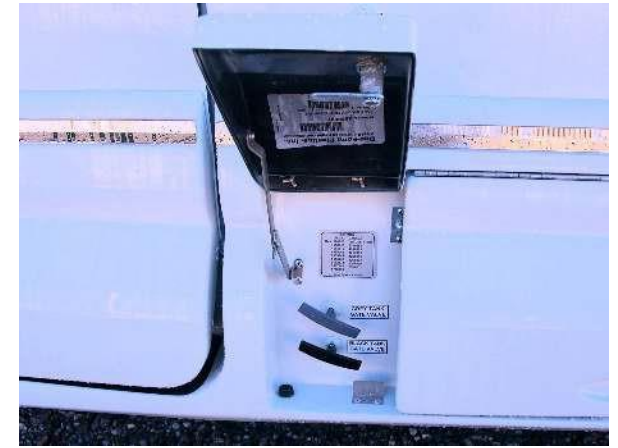
Driver's side front access door showing tank dump valves
