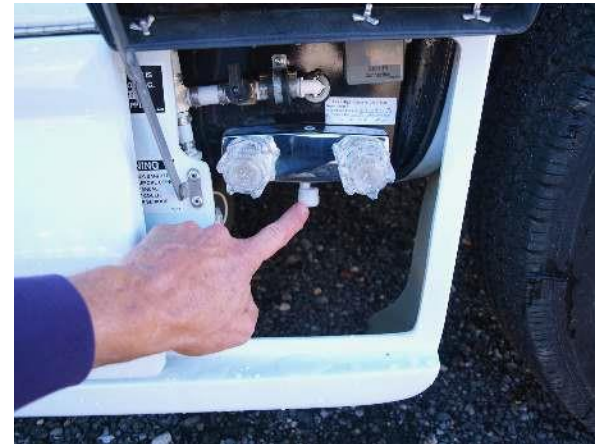
Outside shower connection
