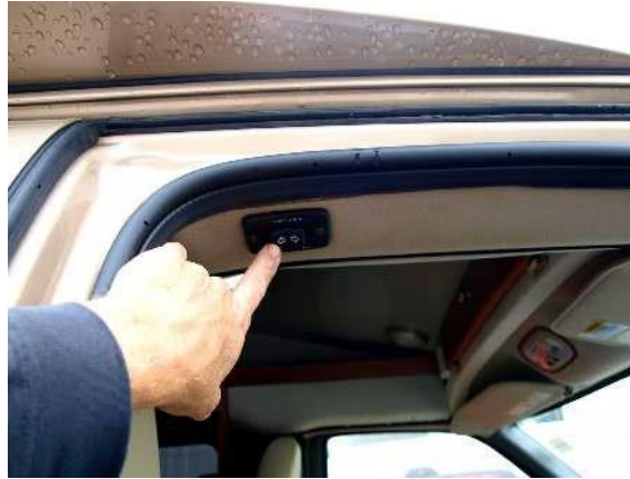
Awning power switch
