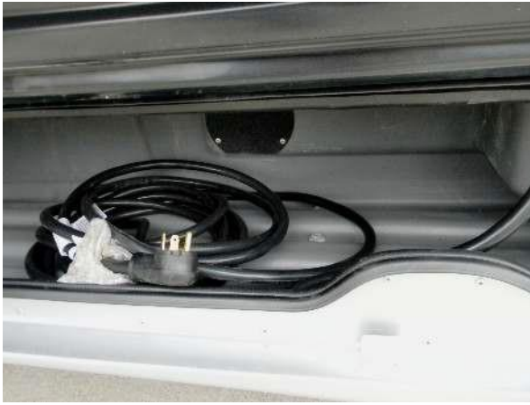
Driver's side center access door houses power cord and waste discharge hose
