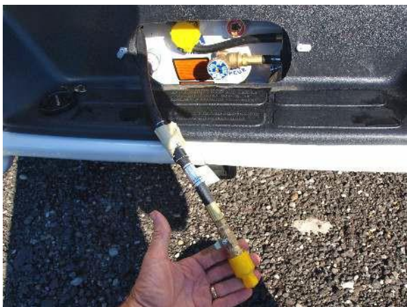
High pressure BBQ pigtail, show with yellow dust-cap and valve in closed position
