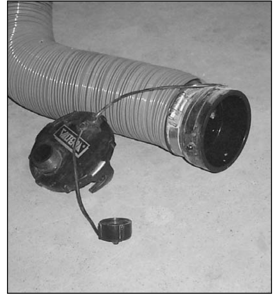
Picture G-P10: Removal of the end cap.
