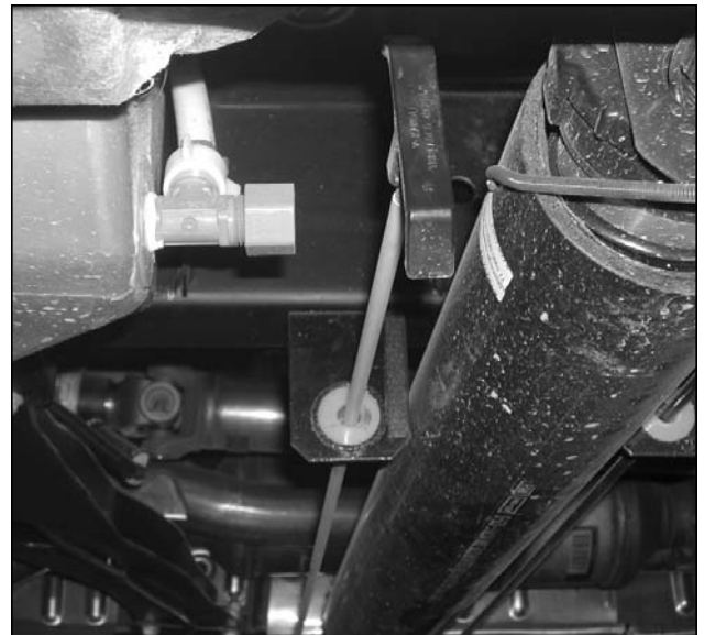
Picture G-P20: Location of the exterior freshwater tank drain.
