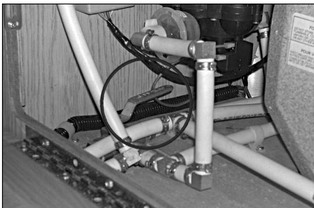
Picture G-P12: The exterior fresh tank transfer line (ball) valve in the open position.
