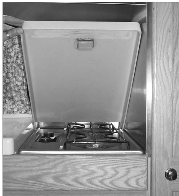
Picture B-P26: Lifting stove counter top
