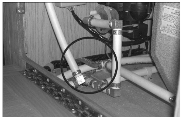
Picture G-P13: The exterior fresh tank transfer line (ball) valve in the closed position.
