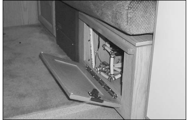
Picture G-P14: Location of the access door for the tank selector valve.
