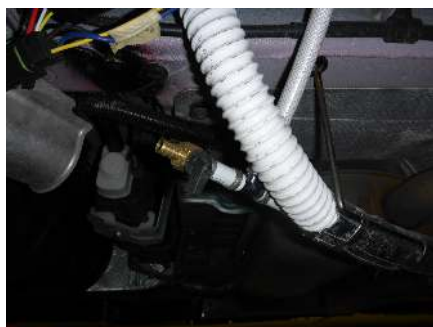
Fresh tank drain under the driver's door
