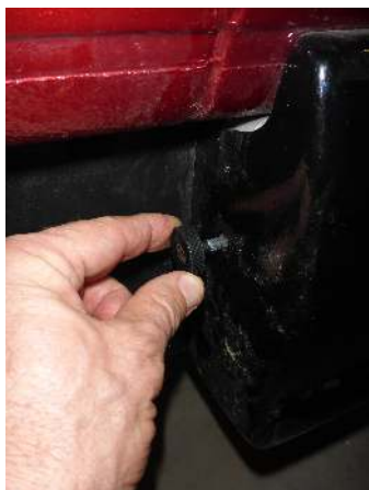
Remove the cover thumb screws
