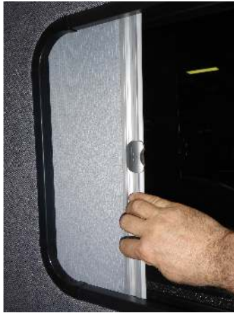
The side window screens - nightshade side
