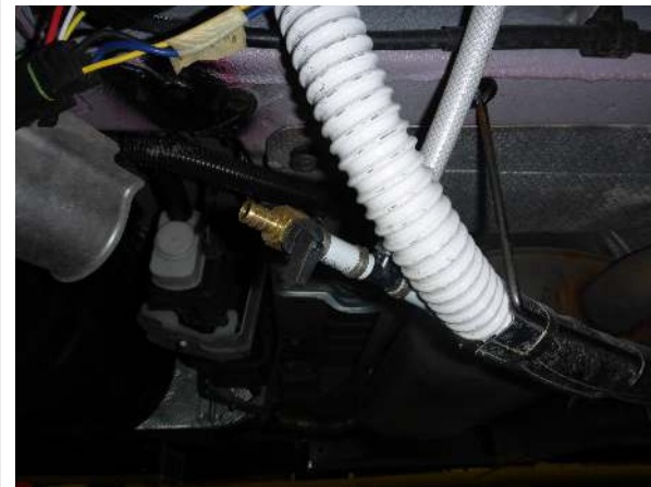
Fresh water tank drain, under driver's doorstep
