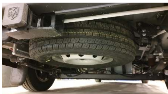
The spare tire is located behind the rear bumper
