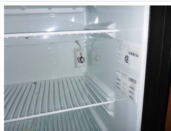
Thermostat is located inside on the rear wall
