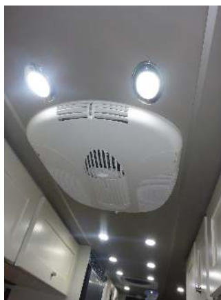
Roof-mount air conditioner
