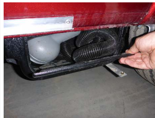
Waste water hose storage
