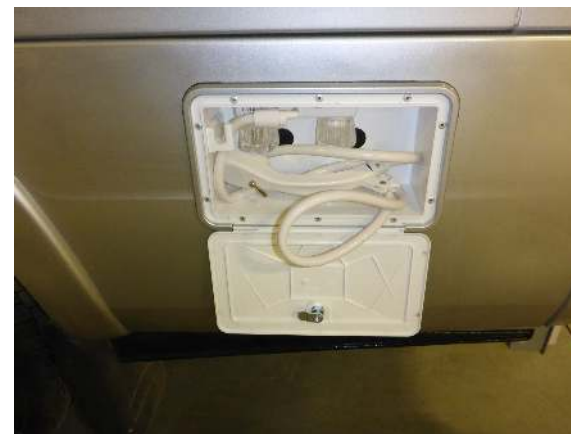
Rear compartment with outside shower faucet
