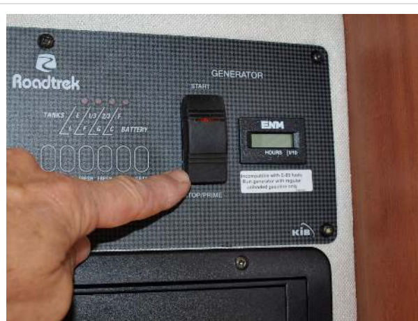
Generator switch, prime/off position
