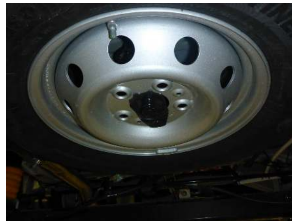
The spare is held in with a positive engagement spring.
