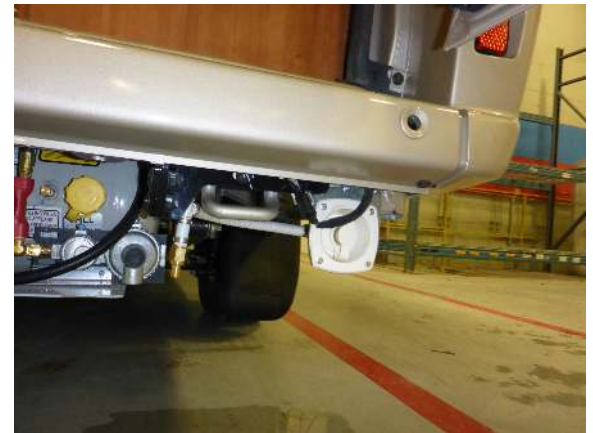
City water connection
