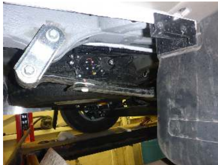
The lowering mechanism is behind the passenger side rear wheel
