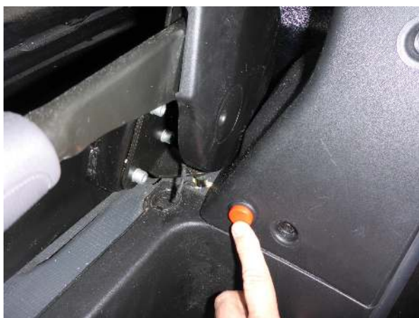
Macerator switch on driver's side doorstep
