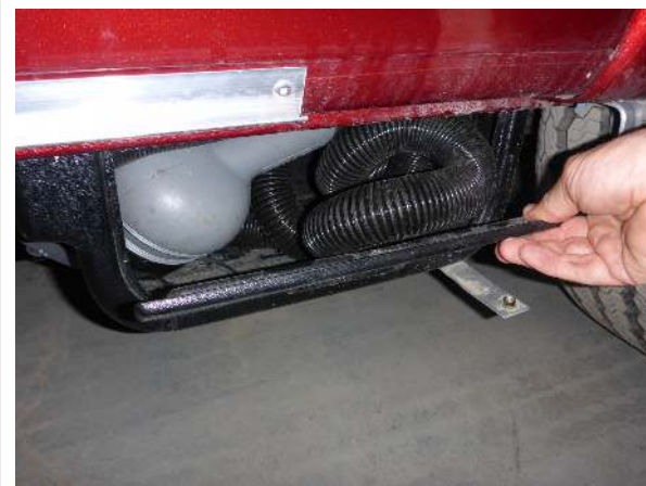
Waste water hose in stowed position
