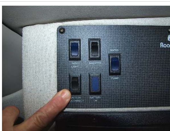
Battery disconnect switch
