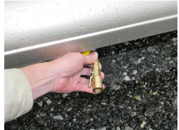
With yellow dustcap removed and valve in open position
