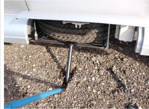
Lower tire carrier to the ground and remove tire
