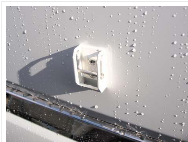
Awning support attachment point
