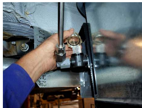
Water pump filter. View is from centerline of vehicle back toward passenger side rear corner.
