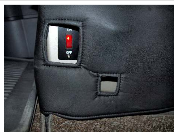
Switch for engine preheat
