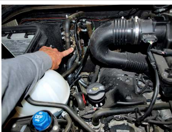
Heat exchanger on engine compartment firewall
