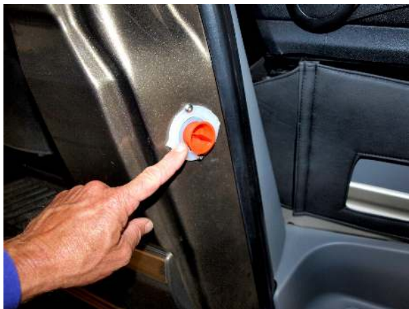
Gravity fill in passenger doorframe
