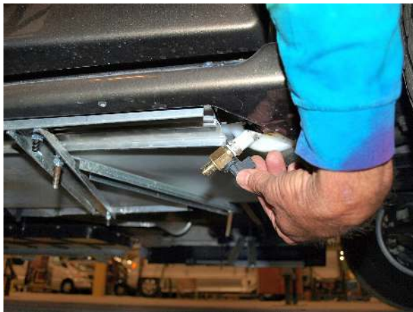
Fresh water tank drain, under passenger front door step
