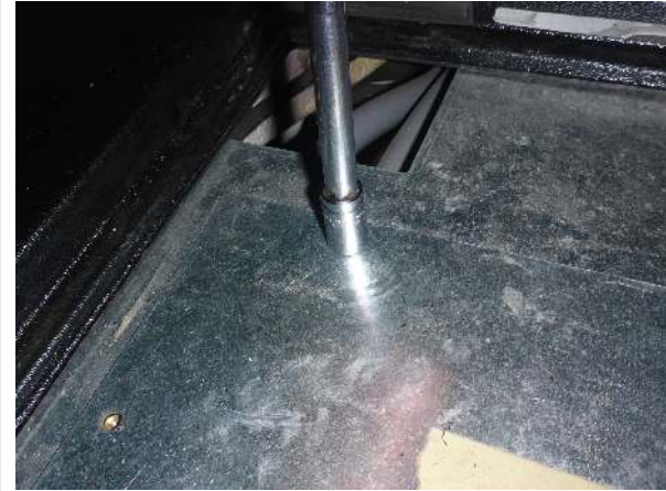
Remove 8 screws and lift up metal cover
