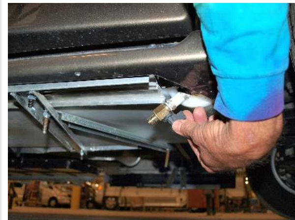
Drain for fresh water tank, under the passenger door step
