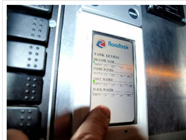
Tank level display
