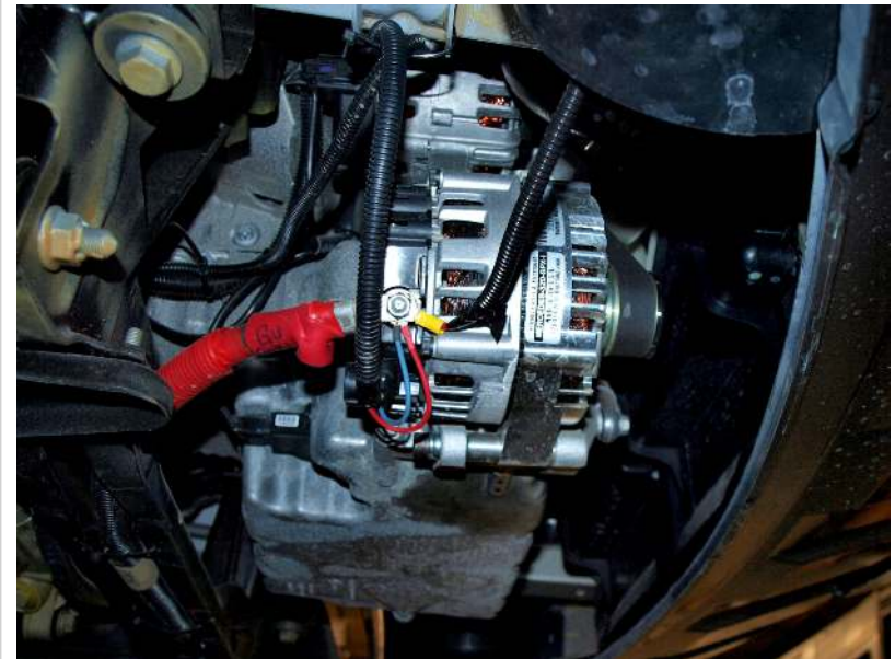
Engine generator mounted on engine
