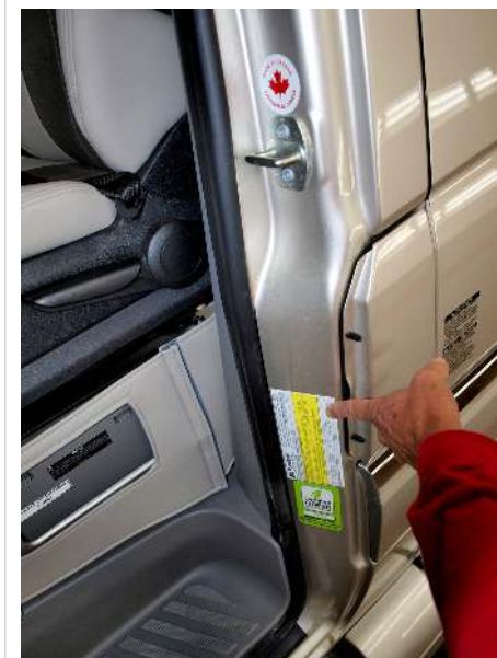
Sticker on driver side B pillar with passenger capacity, chassis weight and tire specs; your sticker will be different
