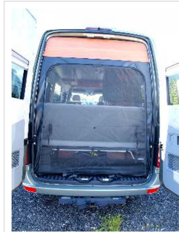
Rear door screen in place
