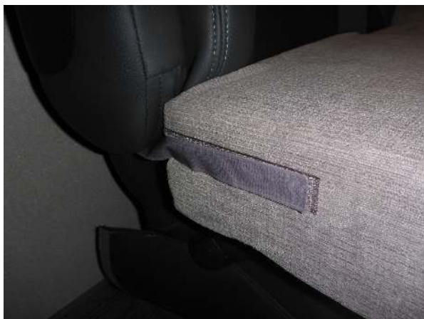
Hook-and-loop strap in place
