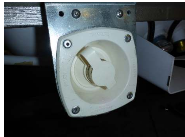
Roadtrek built-in pressure regulator has the words "Water Pressure Regulator" on the plastic collar
