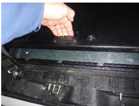
Alde valve access
