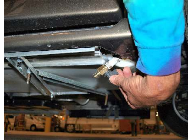
Drain for freshwater tank, beneath passenger doorstep
