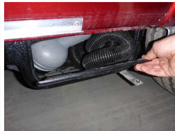
Waste water hose in stowed position
