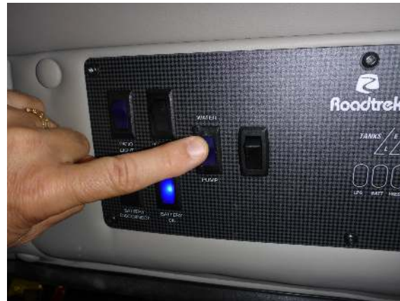
Water pump switch
