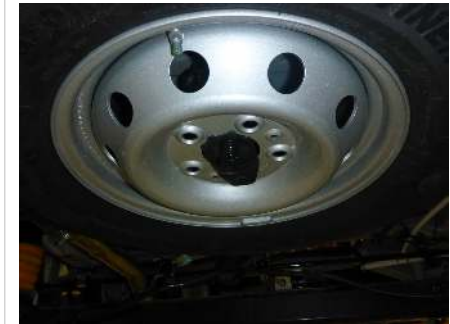
The spare is held in with a positive engagement spring.
