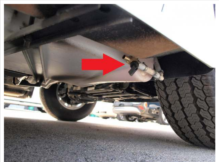
Freshwater tank drain valve
