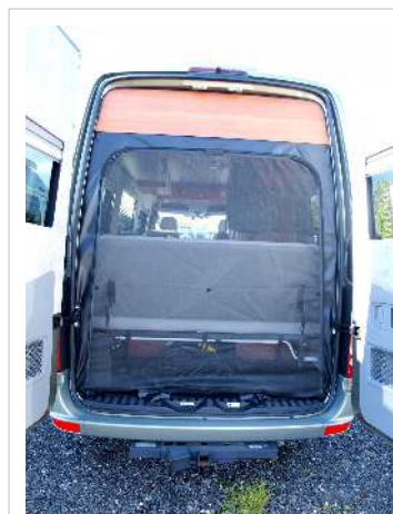
Rear door screen in place
