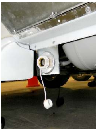
City water fill location
