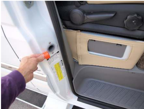
Fresh water gravity fill
