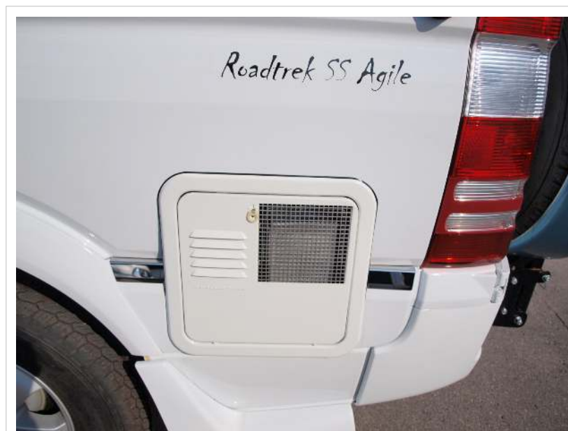
Outside view of the water heater
