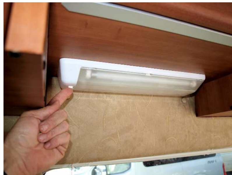
Fluorescent light switch
