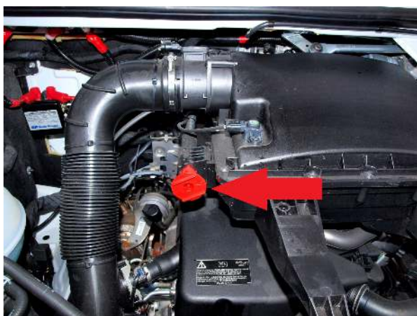
Positive jumper point, on passenger's side of the engine. Push the red disc in to expose the contact.
