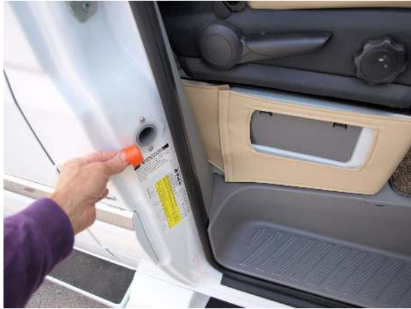
Gravity fill on passenger doorframe
