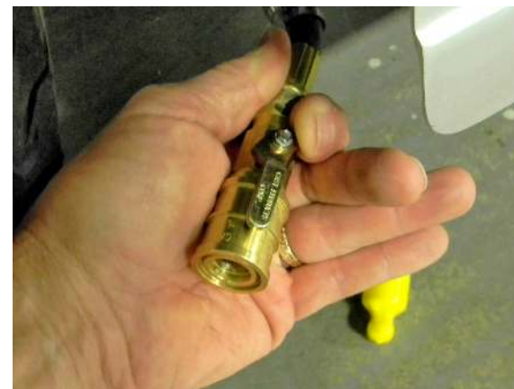
Valve in open position
