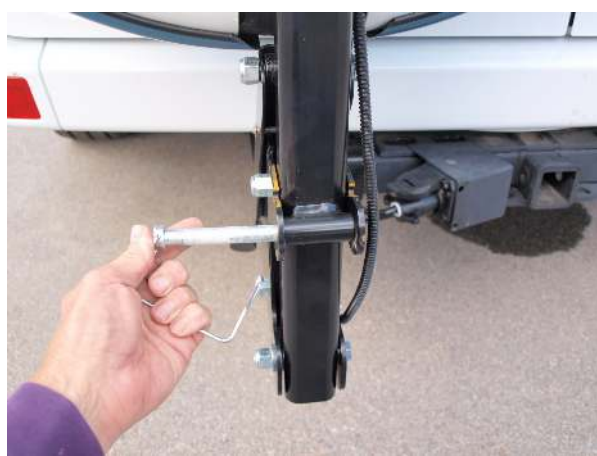
Retaining pin for spare tire carrier
