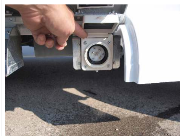
Shore power connection point
