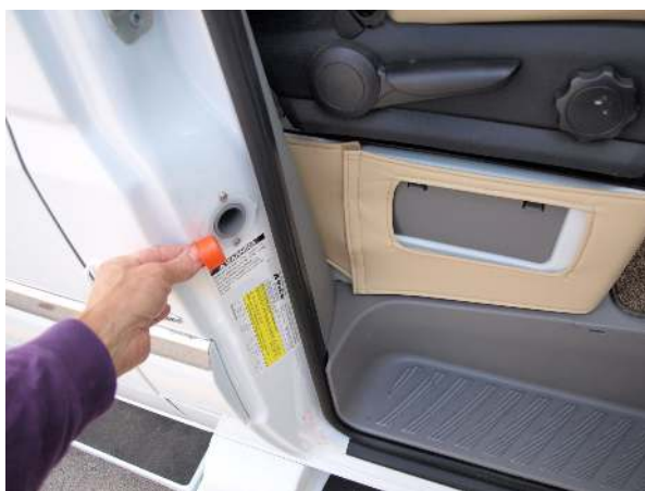
Gravity fill in passenger doorframe
