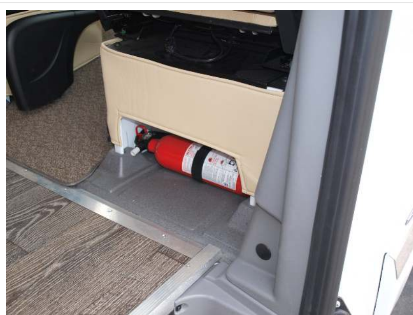
Fire extinguisher located under front passenger seat
