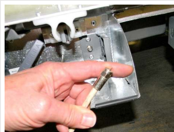
Coaxial TV connecting wire with screw-on end
