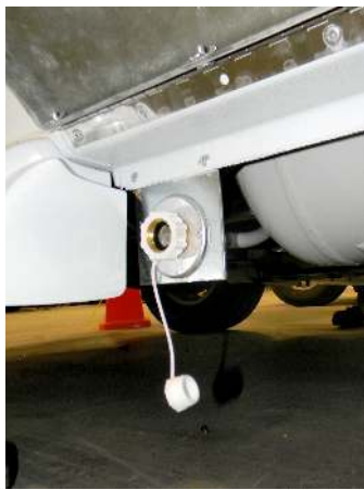
City water fill location
