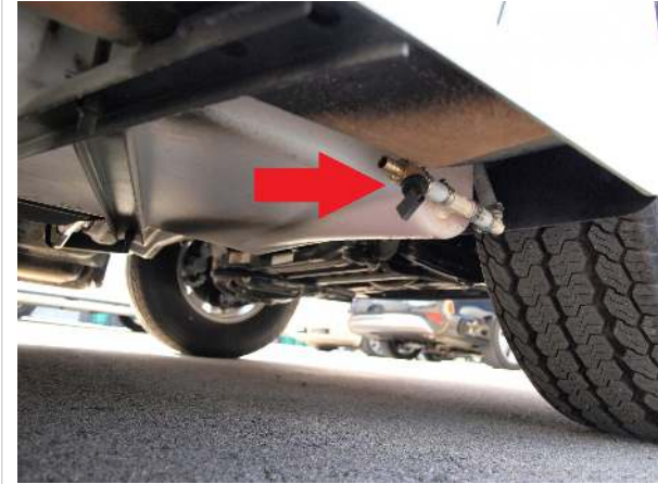
Drain for freshwater tank, beneath passenger doorstep
