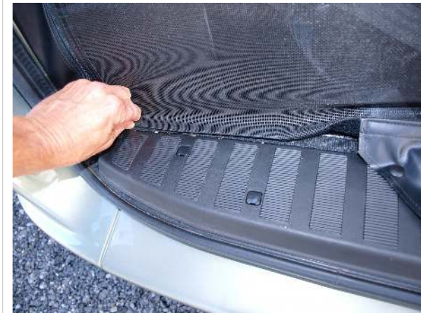
Rear screen lower hook-and-loop fastener
