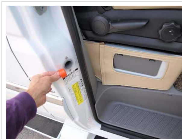
Gravity fill on front door post
