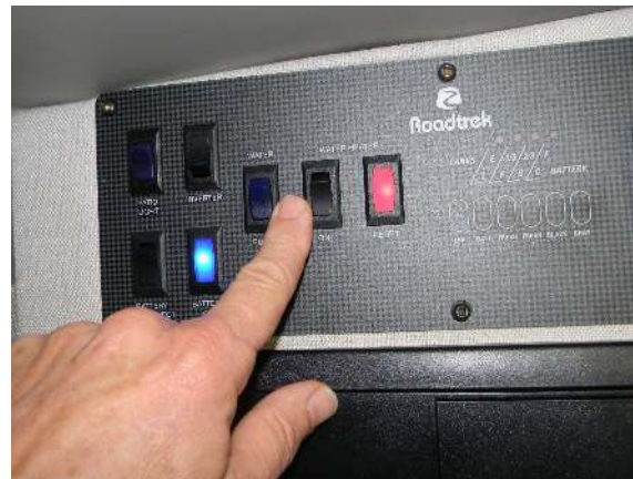
Water heater switch and red indicator light
