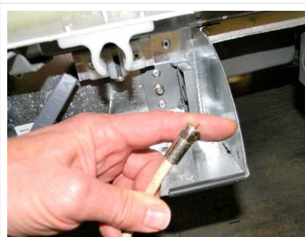
Coaxial TV connecting wire with screw-on end
