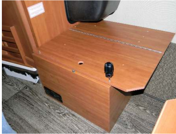
Water pump access inside passenger side bench enclosure
