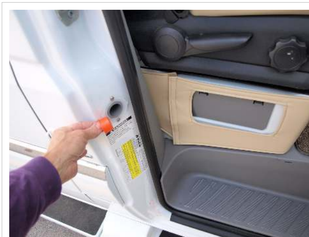
Gravity fill on front door post
