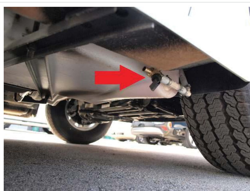
Freshwater tank drain valve
