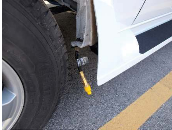
Propane connection with dustcap
