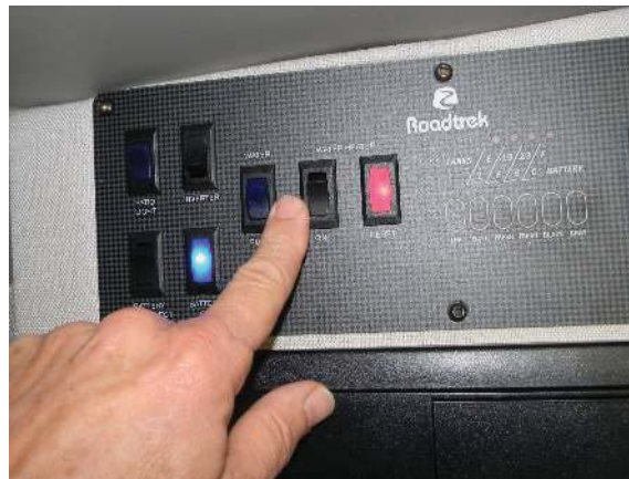
Water heater switch and red indicator light
