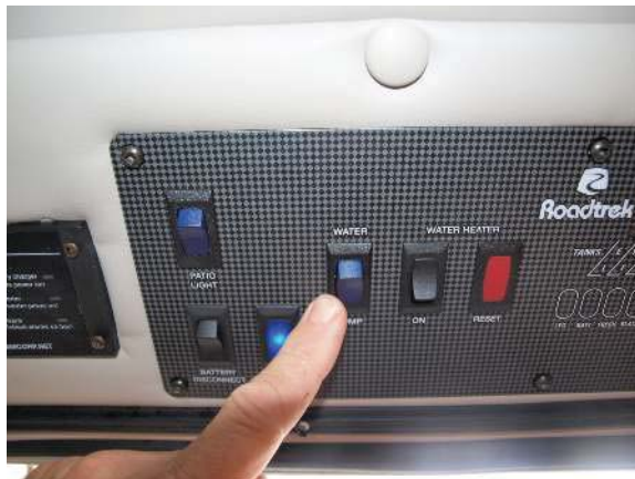
Water pump switch
