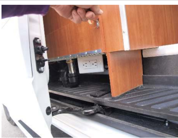
Access to city water valve
