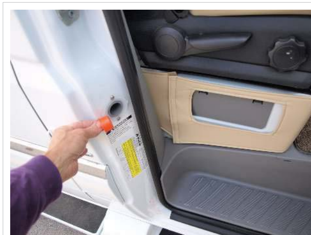
Gravity fill on front door post
