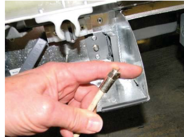
Coaxial TV connecting wire with screw-on end
