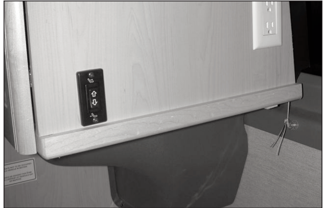
Picture B-P10A: Location of the power rear sofa remote switch.
