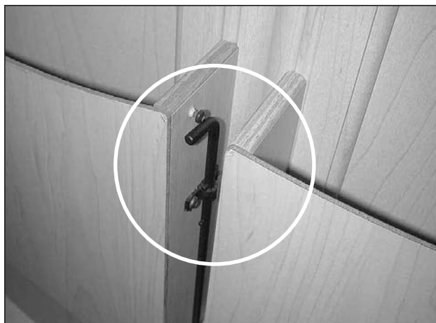
Picture B-P21: Front bathroom door, (in transit) locking pin in the locked position.
