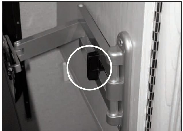
Picture B-P28: Flat screen display bracket locking "T" handle.
