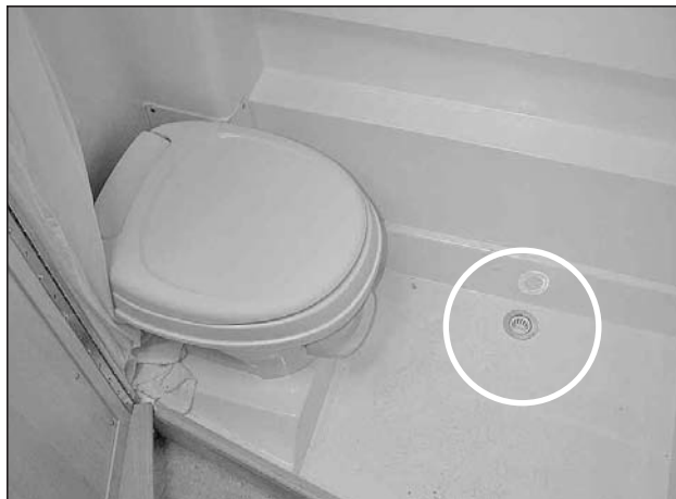
Picture B-P24A: Location of permanent bathroom shower drain.
