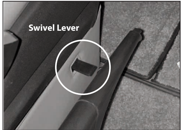
Picture B-P1: View of front captain's seat showing the location of the swivel lever.
