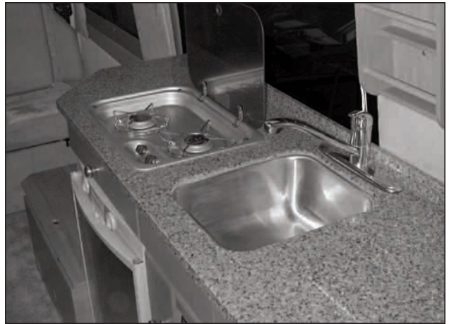
Picture B-P26: Counter top with sink cover removed and stove cover open.
