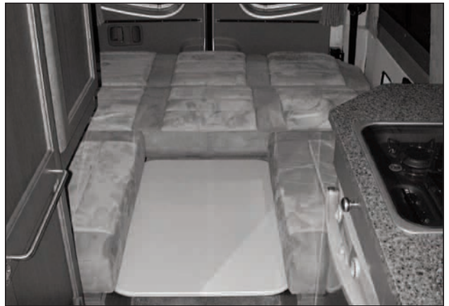
Picture B-P11A: Placement of the table top as the center bed support for the king size bed.
