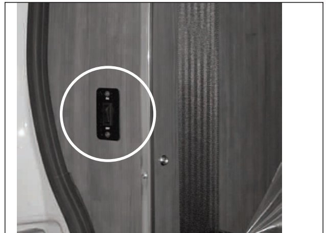
Picture E-P2: Location of the porch light switch (RS model).
