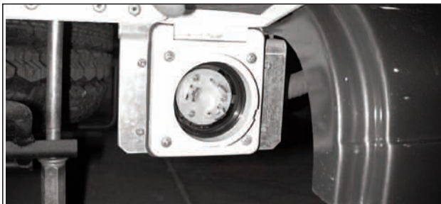
Picture B-P33: Location of exterior shore power connector (RS model shown).
