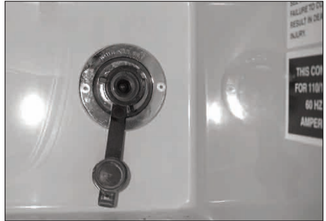
Picture G-P0: City water fill check valve (in very center of city fill connector).
