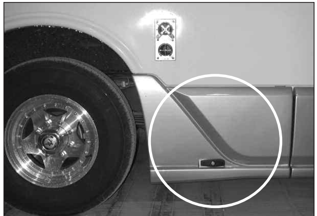
Picture B-P42: Auxiliary battery compartment.
