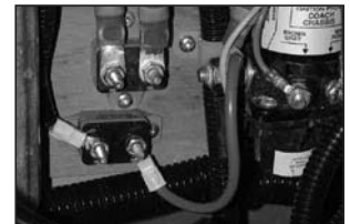
Picture B-P26A: Power Sofa 30A breaker
