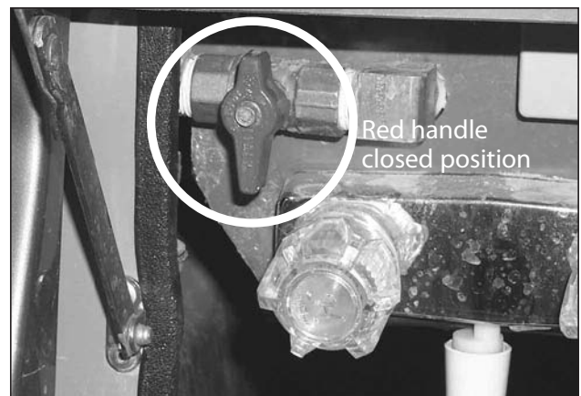
Picture G-P5: Closed position of the city tank fill valve. (Valve may not be exactly as shown)
