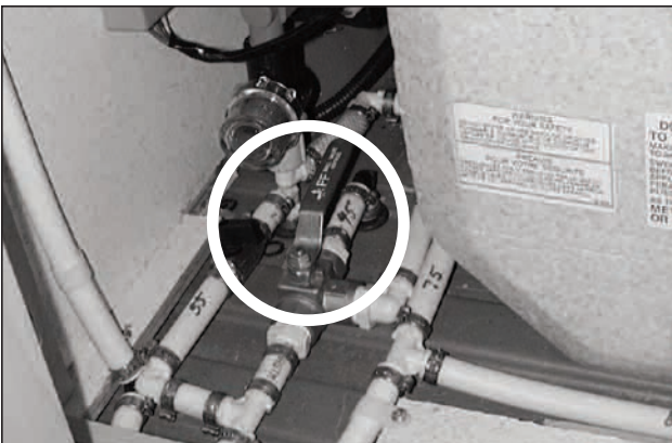
Picture G-P12: Selector valve set to exterior fresh water tank, (summer mode 190 models). NOTE: Water flow is opposite to markings on handle.
