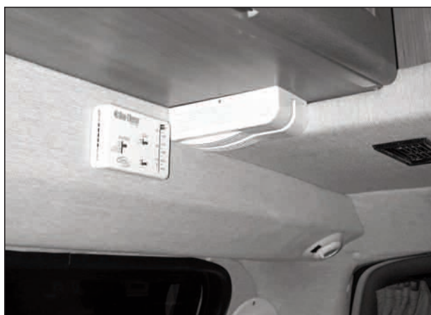
Picture F-P2: Carbon monoxide leak detector, (All models).
