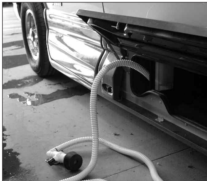
Picture G-P10: Macerator hose location
