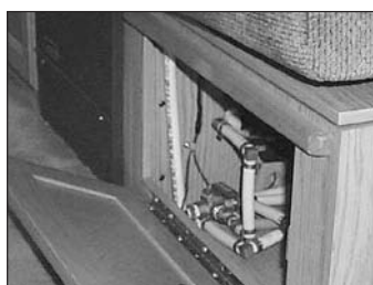
Picture G-P16: Location of the access door for the fresh water selection tank valve, (190 model).
