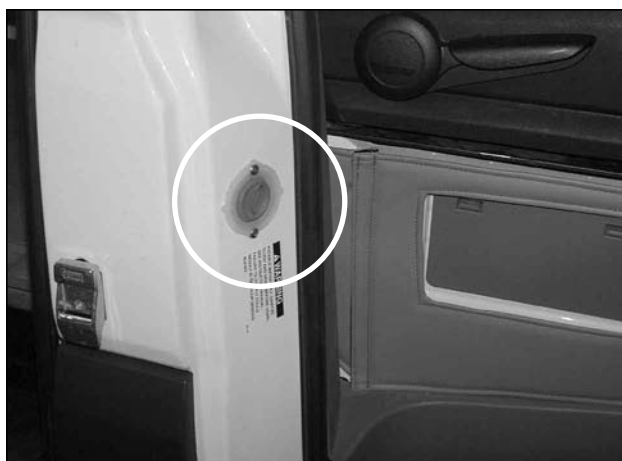
Picture G-P5: The gravity fresh water fill for the fresh water tank, (located on the passenger side front "B-pillar").
