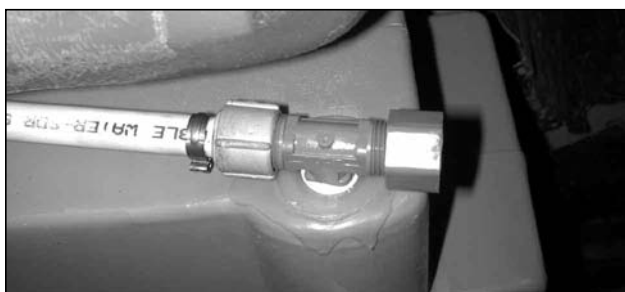
Picture B-P37: Location of the exterior fresh water tank drain cap (visible in passenger front wheel well).
