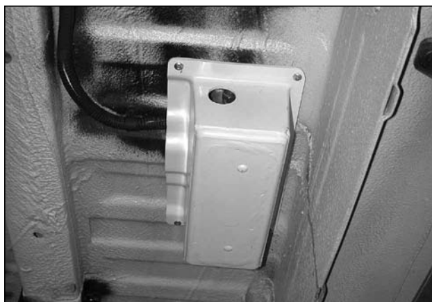
Picture I-P02: Manual crank bolt access. If the hole is offset from the cover (as shown), you will have to remove the cover to access the bolt.
