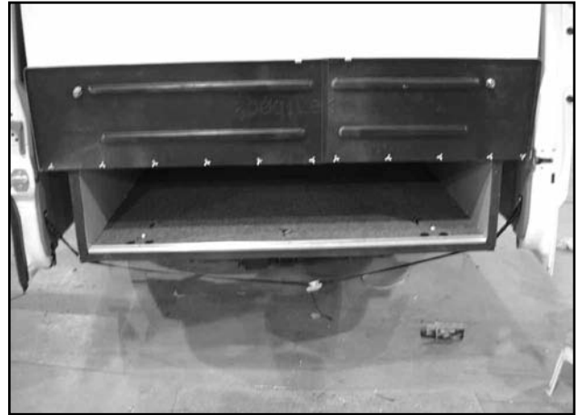
Picture B-P6: Rear doors showing storage area and restraint strap (hanging loose).
