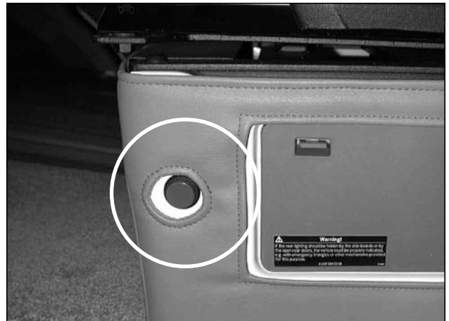
Picture G-P12: Macerator pump switch, (red button) located at the side front of the driver seat pedestal.
