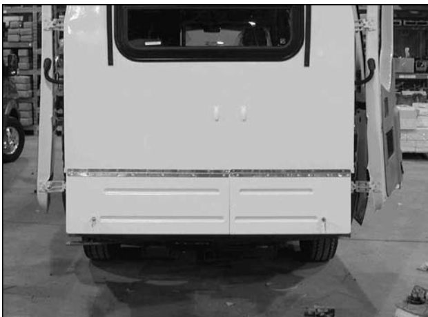
Picture B-P41: Storage area in rear of slideout showing split door (shown in closed position).
