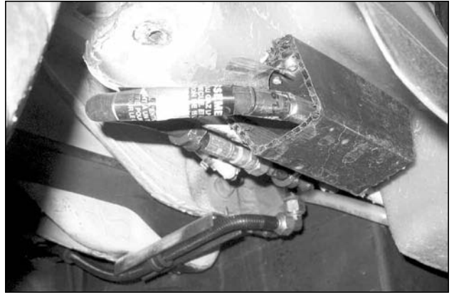
Picture B-P52: BBQ propane supply line in-transit storage location (seen from below).
