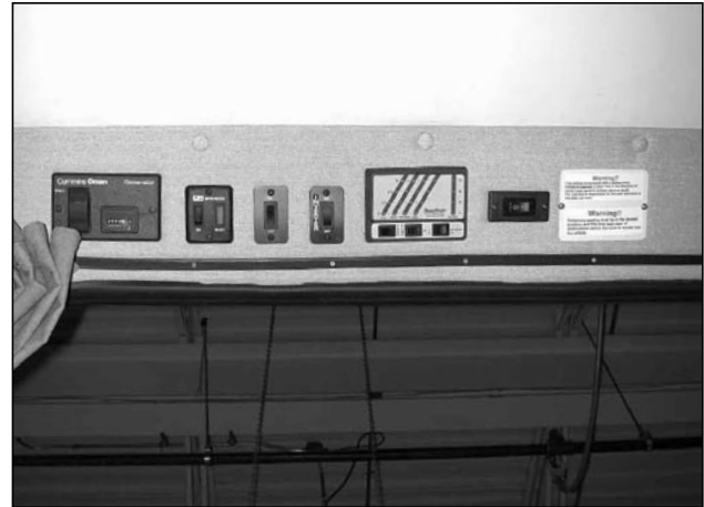
Picture E-P5: Monitor panel, water heater switch, inverter remote switch, porch light switch (SS model), and optional generator control switch.
