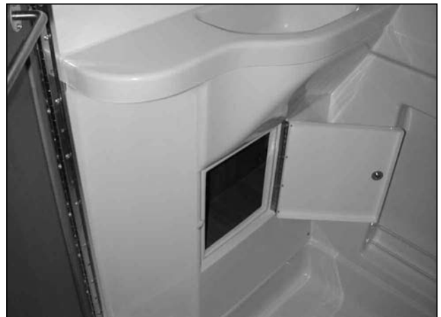
Picture B-P32: Storage compartment in bathroom vanity, (used for storage of extra toilet tissue and other supplies).
