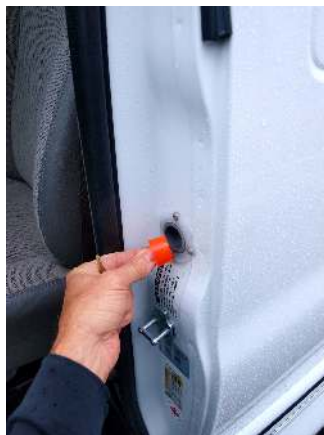
Fresh water tank fill location
