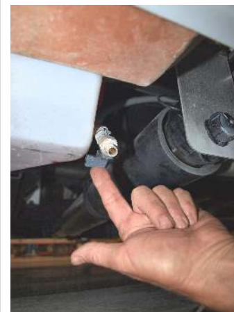
Fresh tank drain
