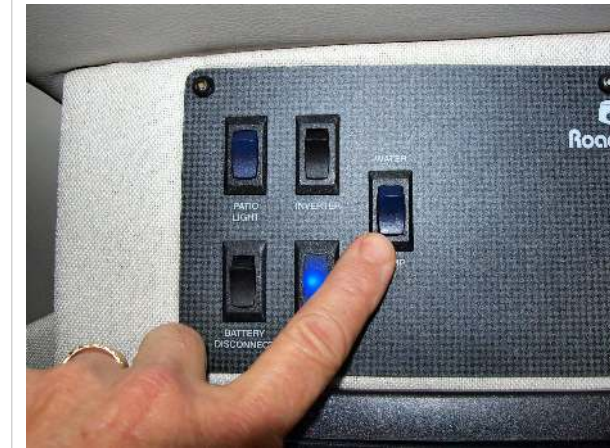
Water pump switch
