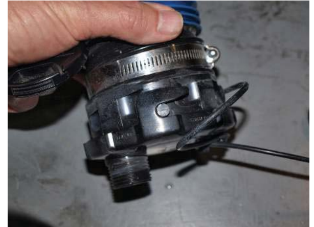
Small cap at end of the hose removed to allow for hose extension
