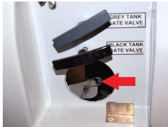
Pin you need to remove to raise the flap and lower the hose pipe
