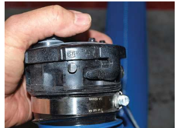
Retaining lugs for hose end - the end has already been twisted open
