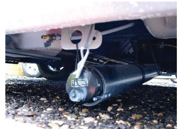
Waste water hose pipe in lowered position
