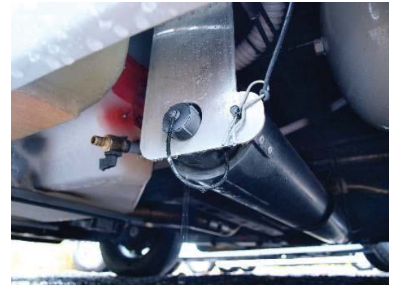
Waste water hose in stowed position
