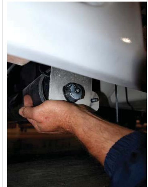
Pushing the wastewater pipe back up - the flap is over the end, and the pin can now be put through the hole in the rod.
