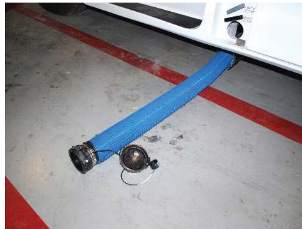
Hose extended toward the dump site
