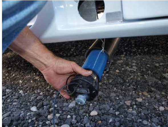
Waste water hose being pulled out of the pipe
