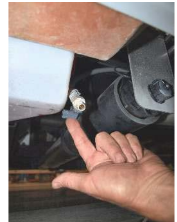
Fresh tank drain
