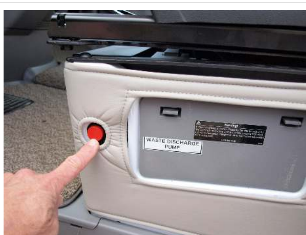
Macerator button on base of driver's seat
