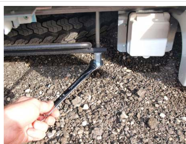
Use supplied wrench to loosen nuts 1/2 inch or so
