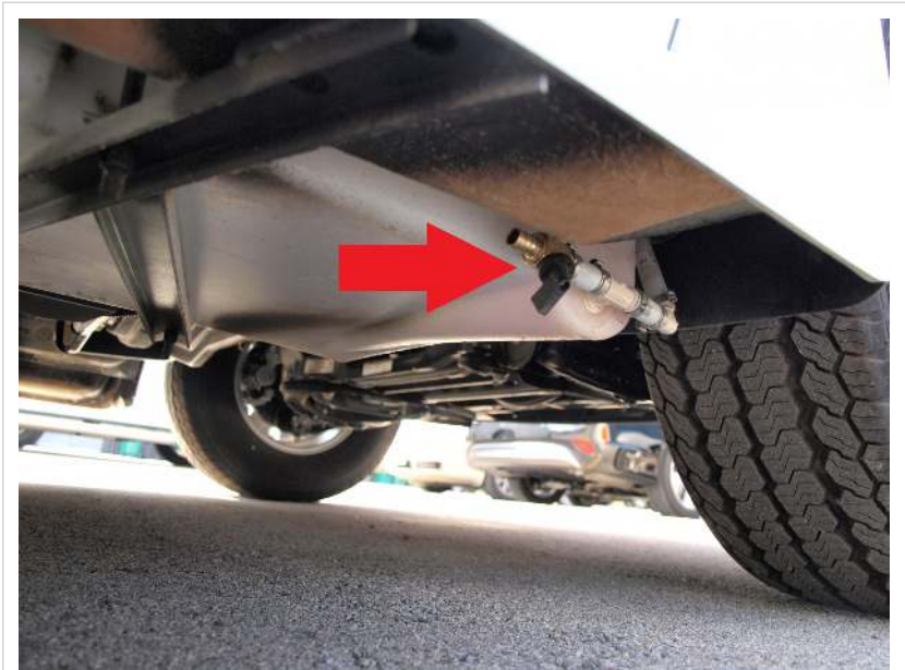
Freshwater tank drain valve
