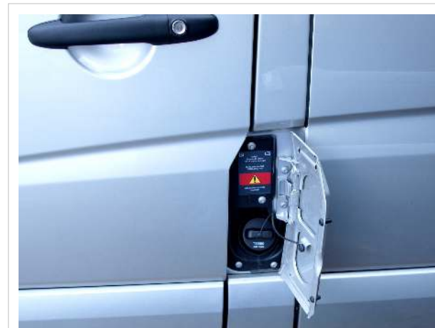
Fuel fill access
