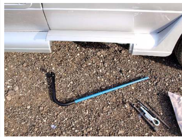
Assembled lever to lower spare tire carrier
