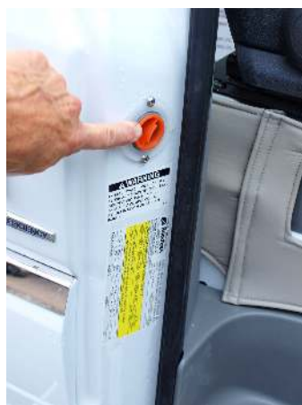
Gravity fill in passenger doorframe
