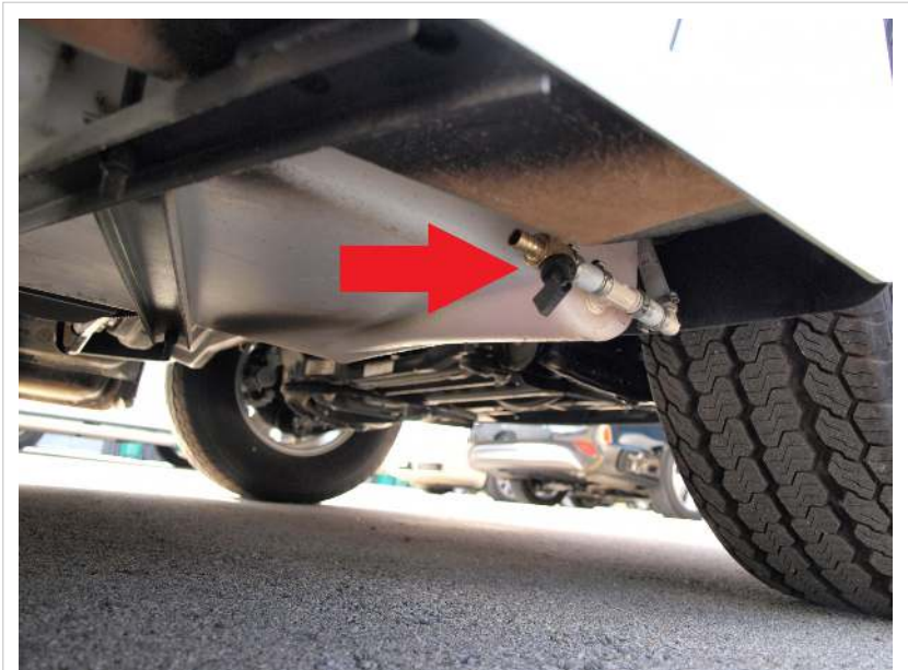
Freshwater tank drain valve
