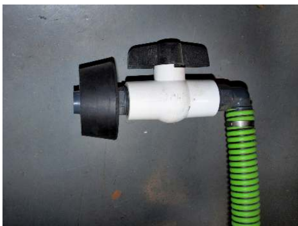
Doughnut installed on nozzle
