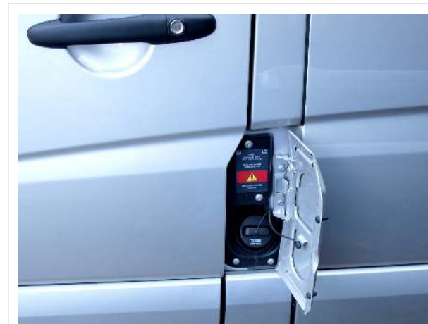
Fuel fill access
