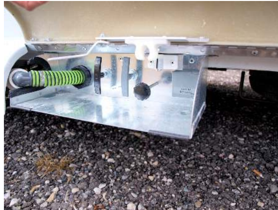
Waste disposal and cable TV access
