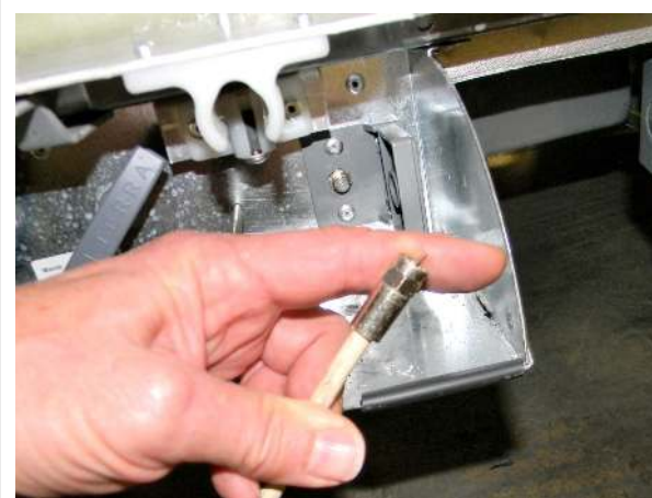
Coaxial TV connecting wire with screw-on end
