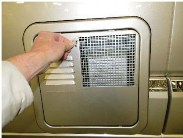
Water heater cover removal (turn tab vertically to remove cover)
