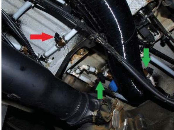
Shunt and Webasto supply line valves in normal position (shunt closed, supply valves open)
