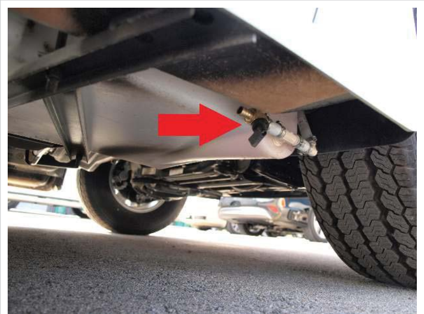
Freshwater tank drain valve
