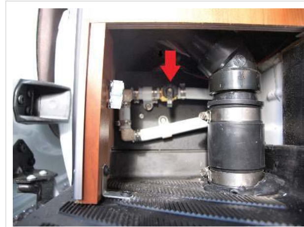
City water valve in closed position (handle across line)
