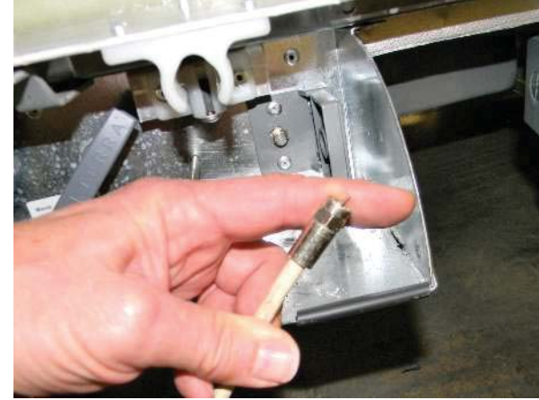
Coaxial TV connecting wire with screw-on end
