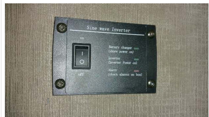
Inverter Control Panel
