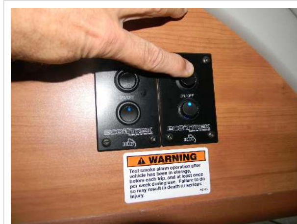
Jump starting an EcoTrek 200; note the left bank is off
