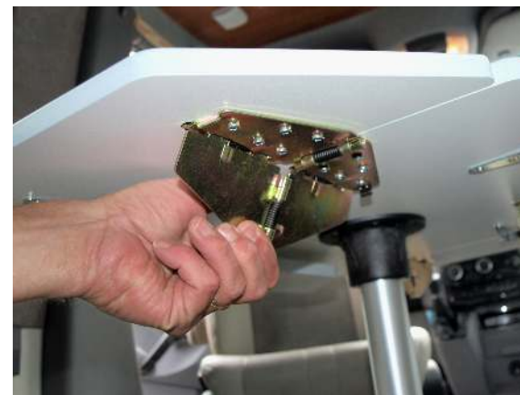
Front table leaves mechanism
