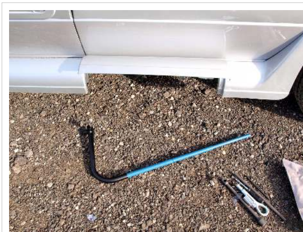
Assembled lever to lower spare tire carrier
