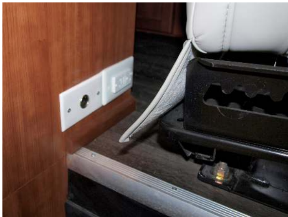
GFCI plug behind rear captain's seat
