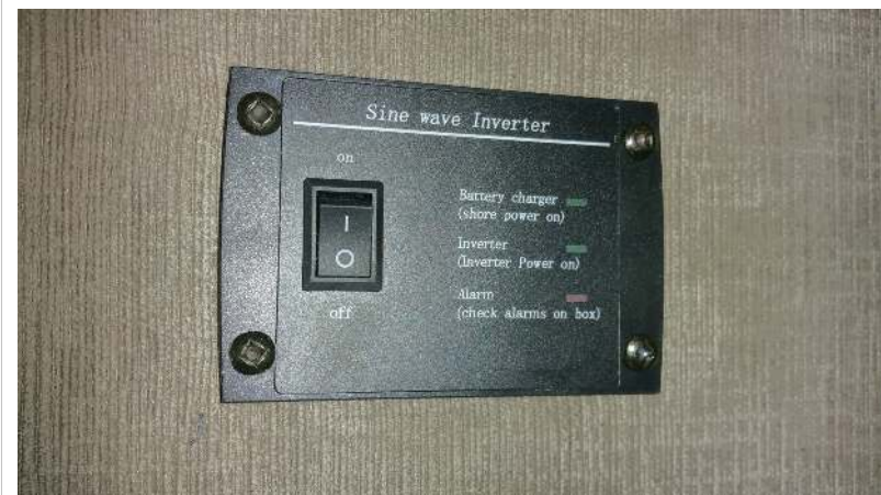
Optional 2500 watt inverter switch
