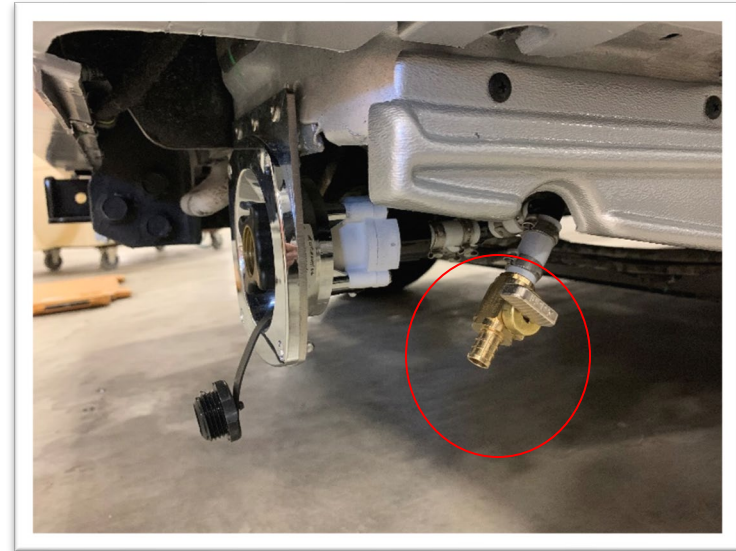
Rear drain behind the city water connection.
