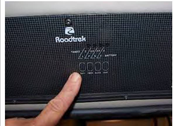
Tank and battery level indicators
