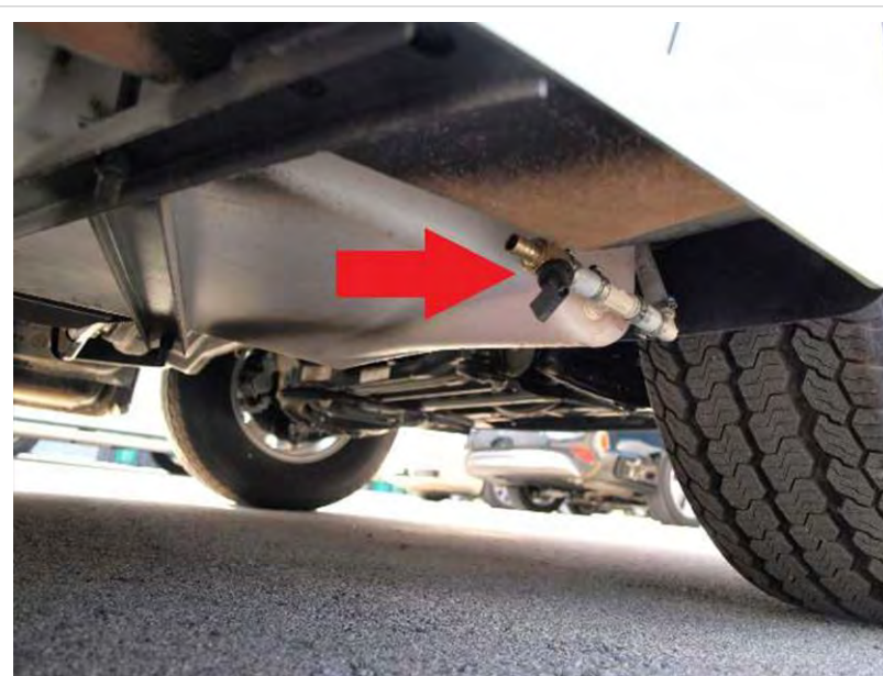
Freshwater tank drain valve
