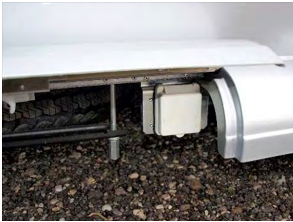
Shore power connection point
