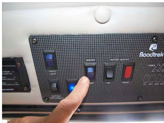
Water pump switch
