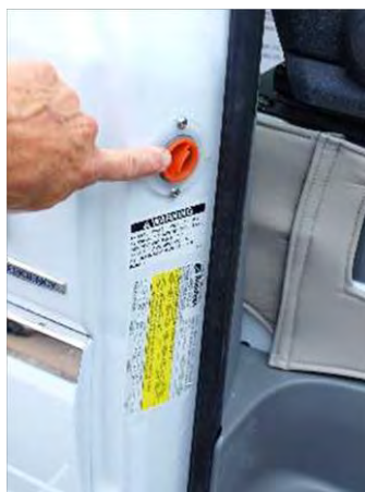
Gravity fill in passenger doorframe
