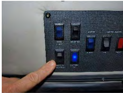
Battery disconnect switch
