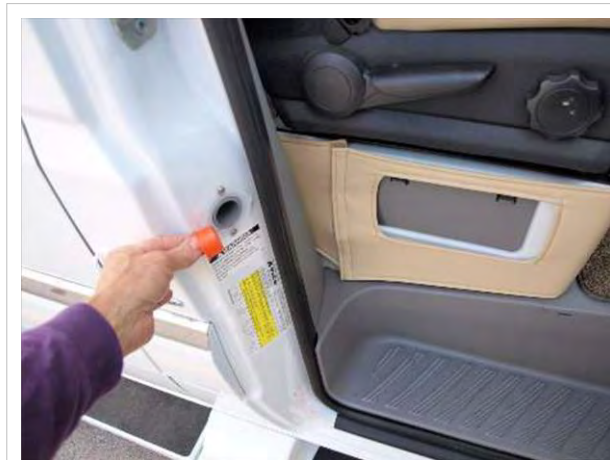
Gravity fill on front door post
