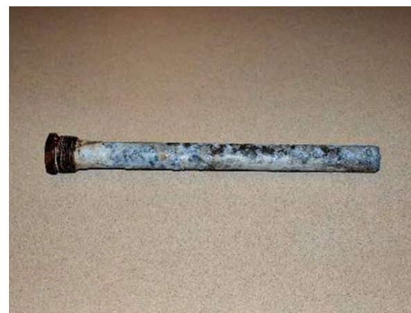
Water heater anode with some corrosion, but probably cleanable and usable for another year.
