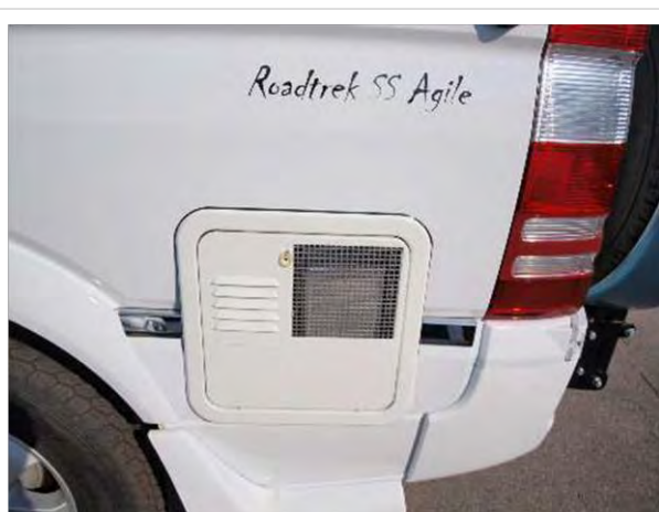
Water heater cover removal (turn tab vertically to remove cover)
