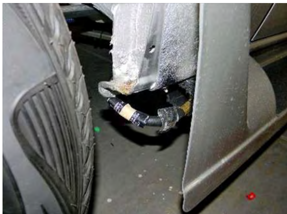
High pressure BBQ connection, in stowed position in front of passenger rear tire
