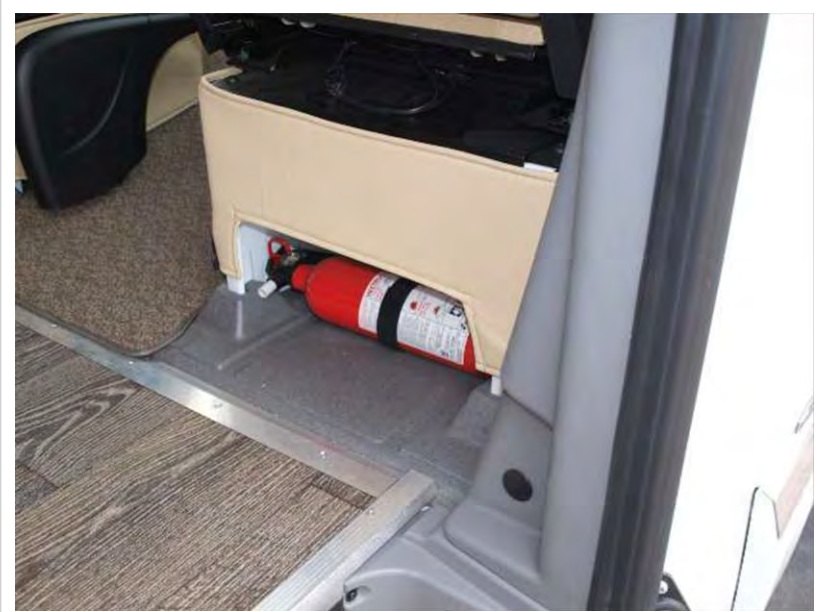
Fire extinguisher located under front passenger seat
