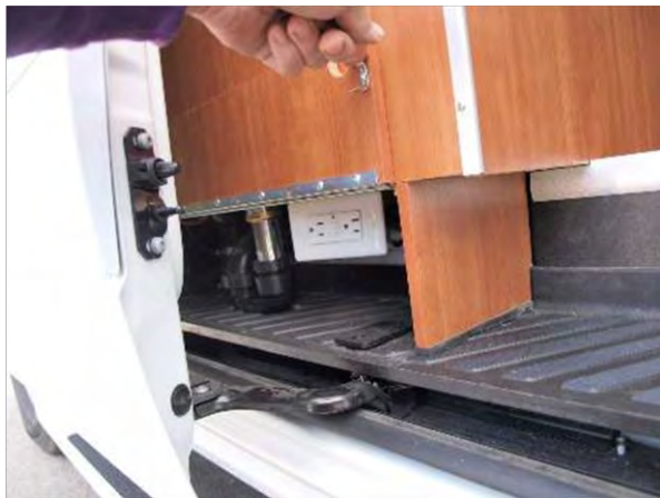
Access to city water valve
