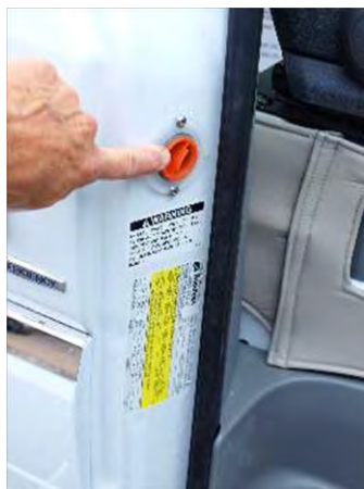
Gravity fill in passenger doorframe
