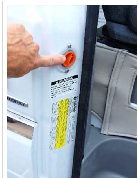
Fresh water fill on passenger door post
