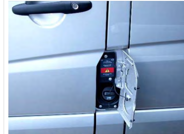
Fuel fill access
