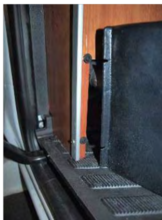
Screws holding plastic radiator cover on
