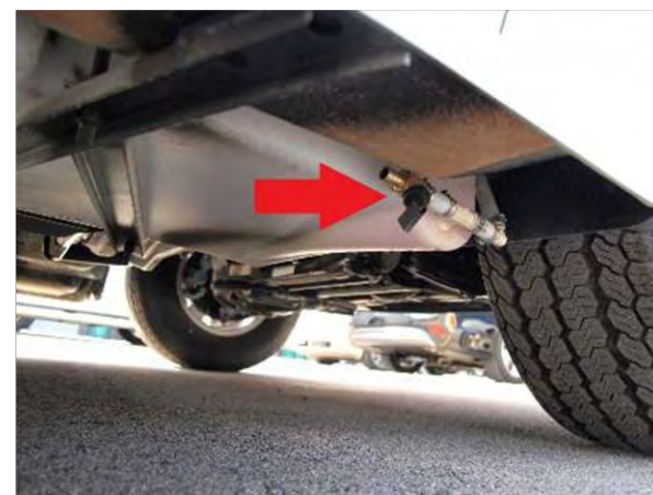
Freshwater tank drain valve
