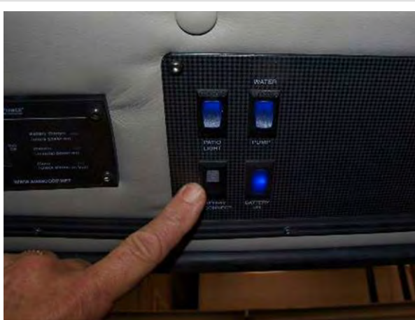
Battery disconnect switch
