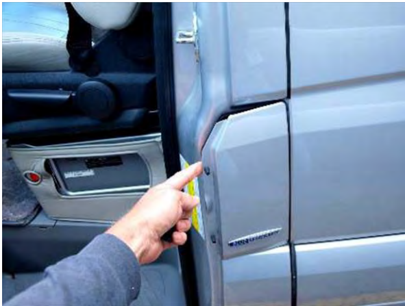
Fuel fill access
