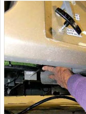
Chevy macerator manual crank knob
