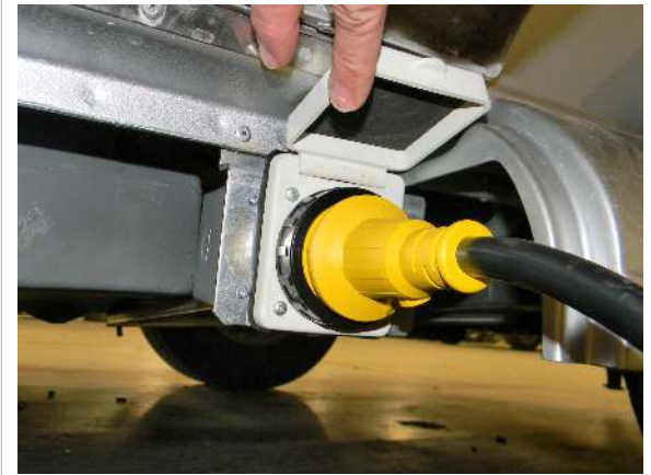
Attached shore power cord
