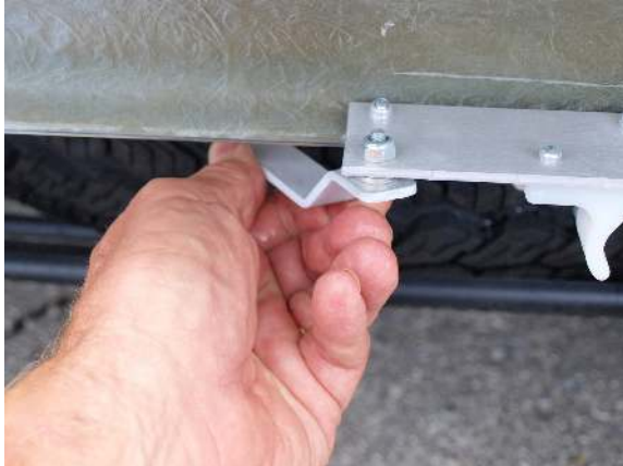
Prop to hold bay doors open
