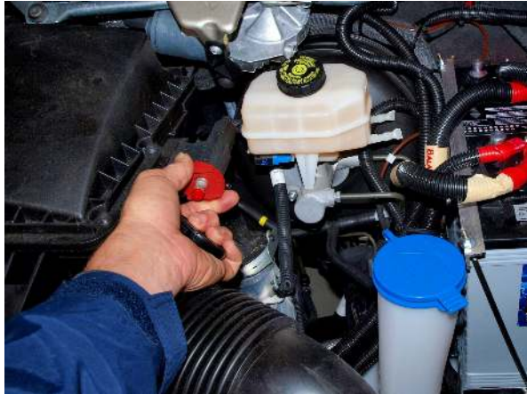
Positive jumper point, on passenger side of the engine. Push the red disc in to expose the contact.
