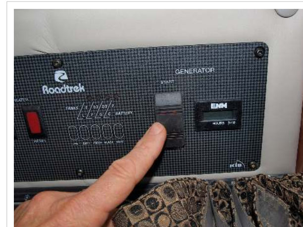
Generator switch and hour meter (optional)
