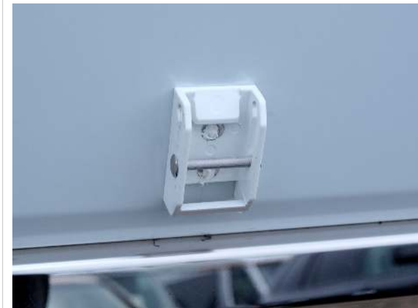
Awning support attachment point
