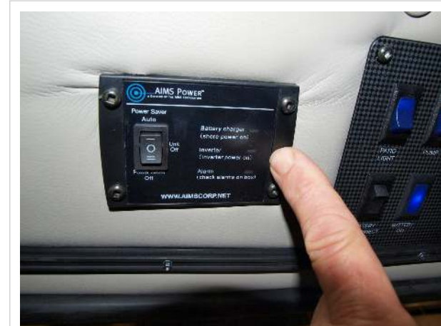
Inverter power indicator light location
