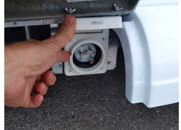
Shore power connection
