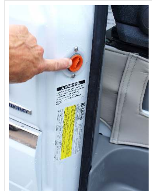
Water tank fill location
