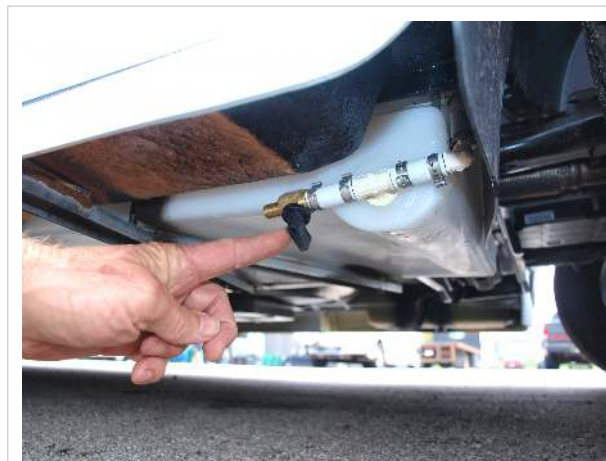
Fresh water tank drain valve
