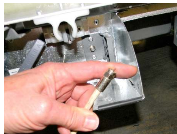
Coaxial TV connecting wire with screw-on end
