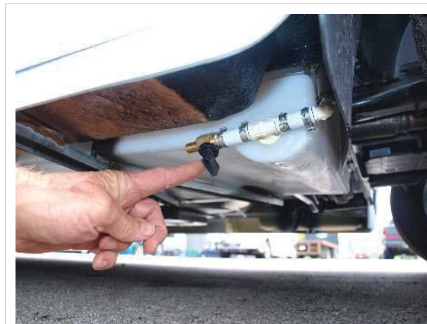
Fresh water tank drain valve
