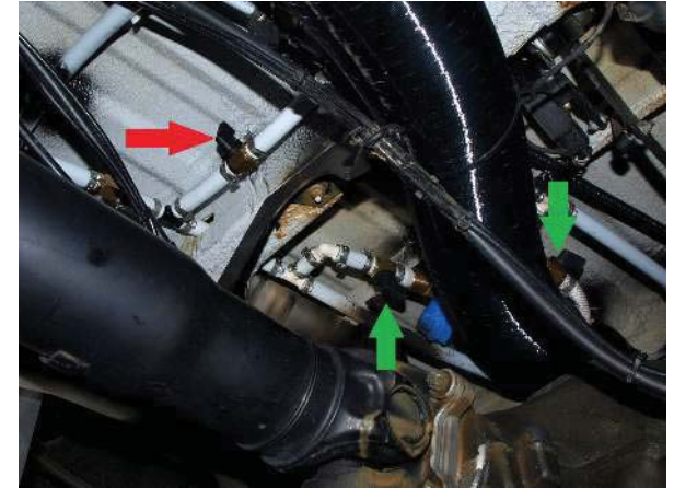
Webasto line valves in normal operating position. Green arrow means valve is open, red closed.
