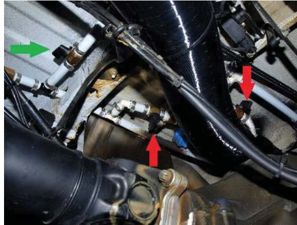
Webasto line valves in bypass position. Green arrow means valve is open, red closed. Front of vehicle is to the upper left.
