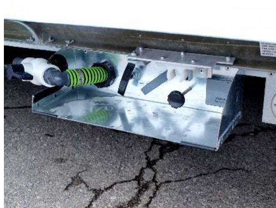
Waste disposal and cable TV access
