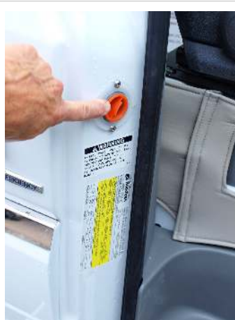
Gravity fill in passenger doorframe
