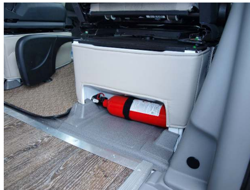
Fire extinguisher located under front passenger seat
