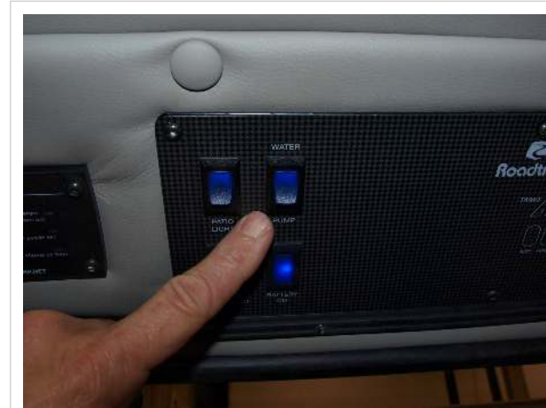
Water pump switch
