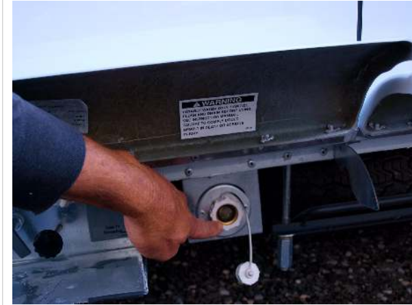
City water connection, driver's side behind access bay door
