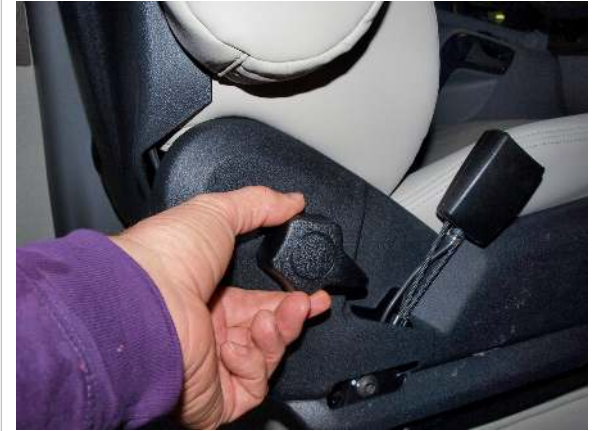
Lumbar support adjustment on inboard side of seat
