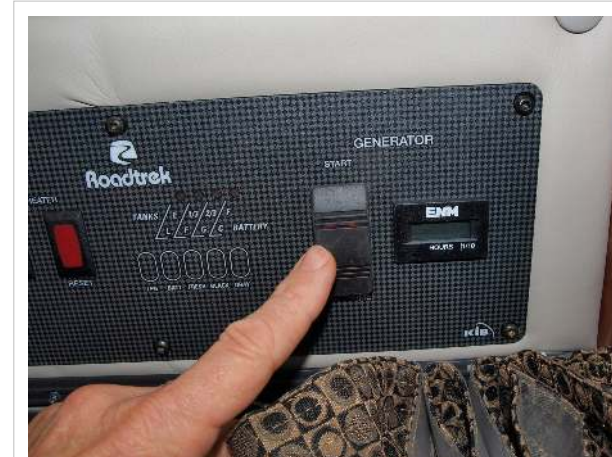
Generator switch and hour meter (optional)
