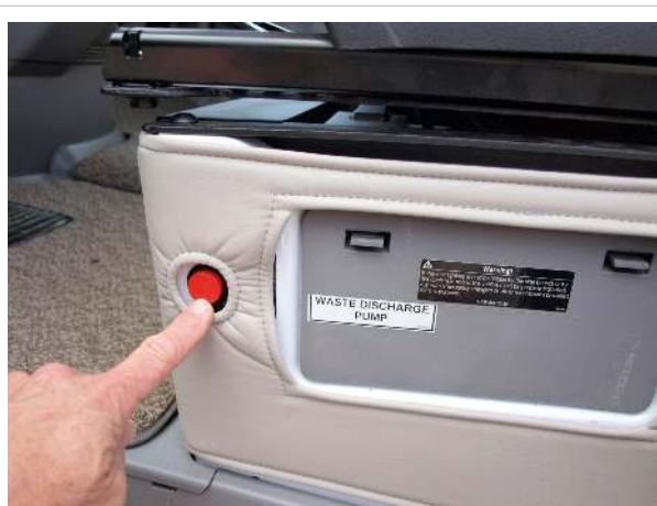
Macerator button on base of driver's seat
