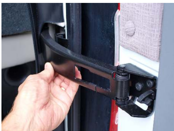
Rear door retaining strap
