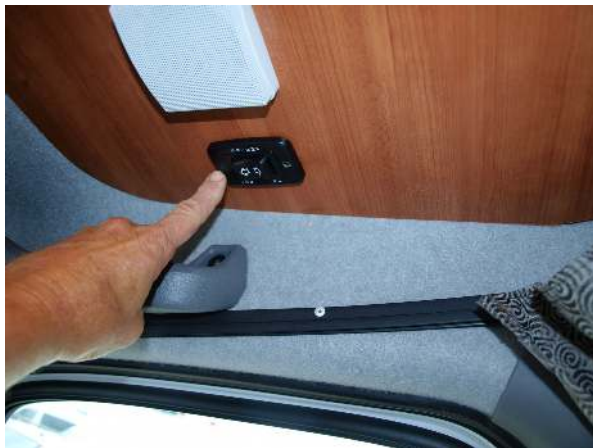
Power awning switch above front passenger seat
