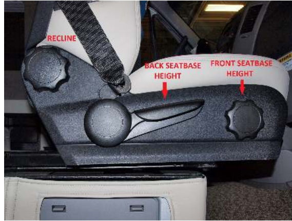
Outboard front seat adjustments
