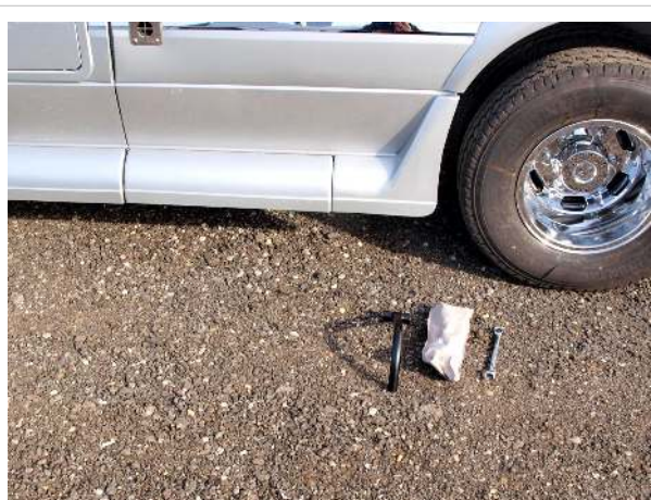
Jack handle pouch and "banana" lever ready to assemble
