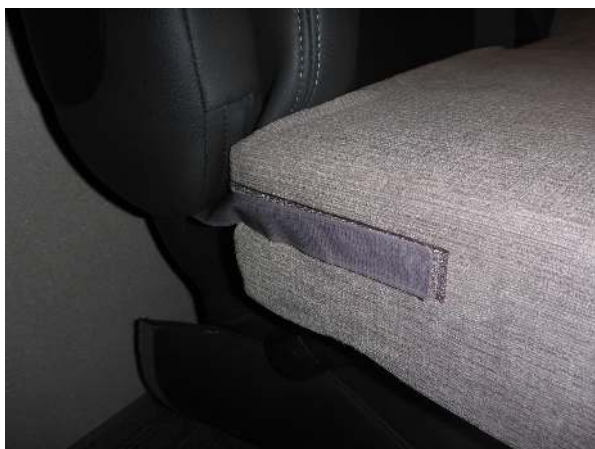
Hook-and-loop strap in place
