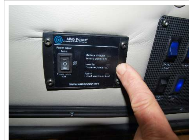
Inverter power indicator light location
