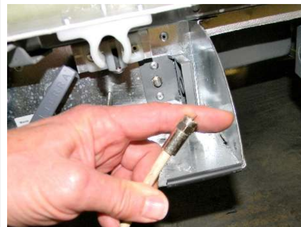
Coaxial TV connecting wire with screw-on end
