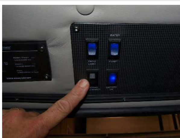
Battery disconnect switch
