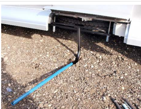
Lever in place to take the weight off the bolts
