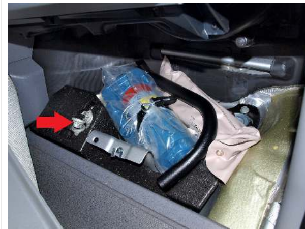
Jack, handle, and "banana" lever to lower spare tire carrier.
