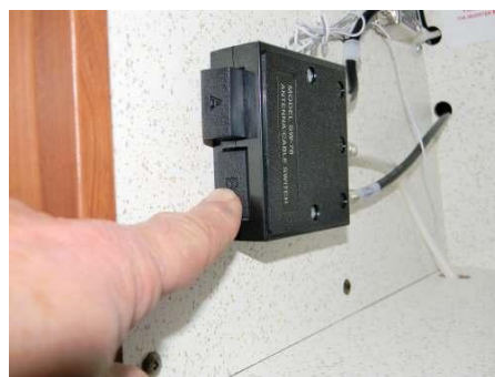
AB switch selected for cable (bottom button)
