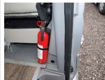
Fire extinguisher located behind front passenger seat
