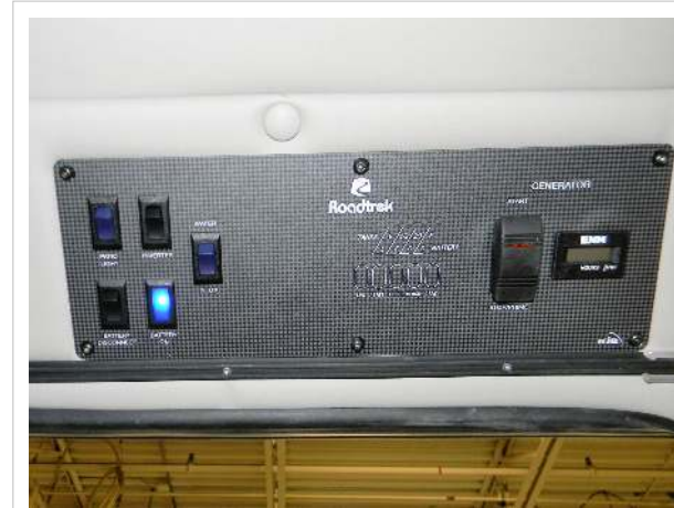
Monitor panel for units with standard 1250 watt inverter and propane generator
