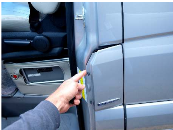
Fuel fill access
