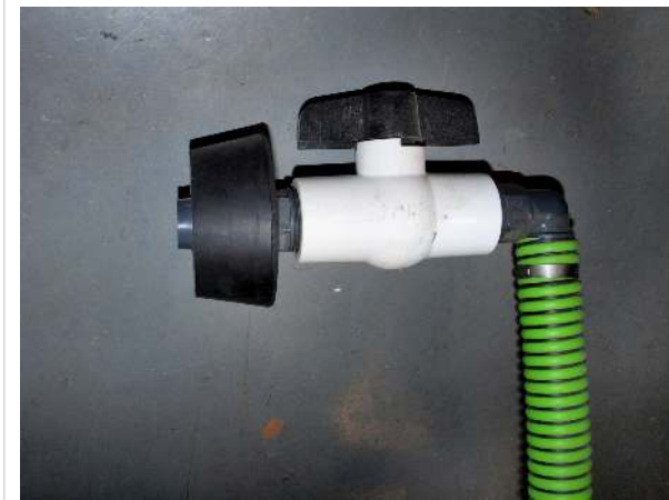
Rubber doughnut installed on nozzle
