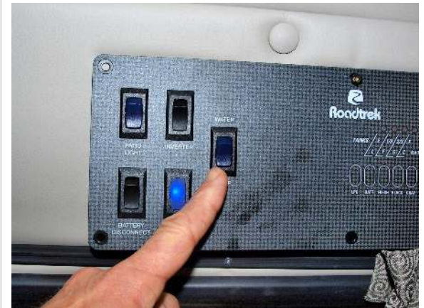
Water pump switch location with standard inverter
