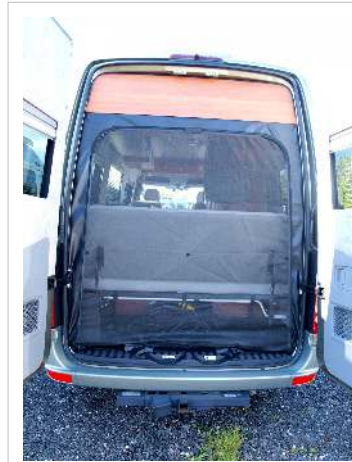
Rear door screen in place
