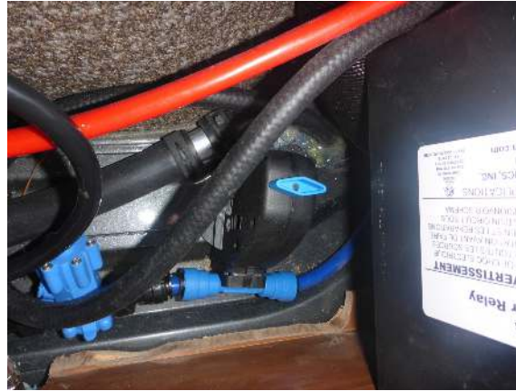
Alde frost protection normal position - blue handle is pointing parallel to the water line, blue button at base is in
