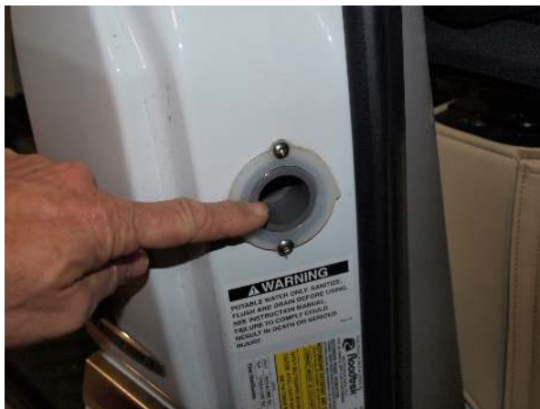
Gravity fill in passenger doorframe
