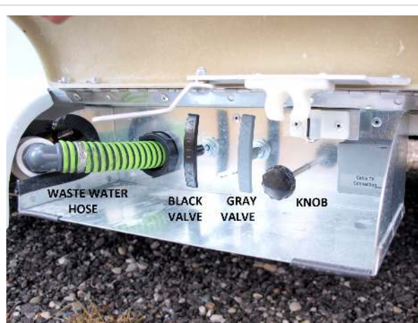
Waste water controls compartment contents
