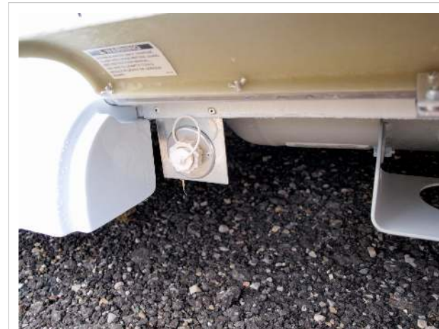
City water connection
